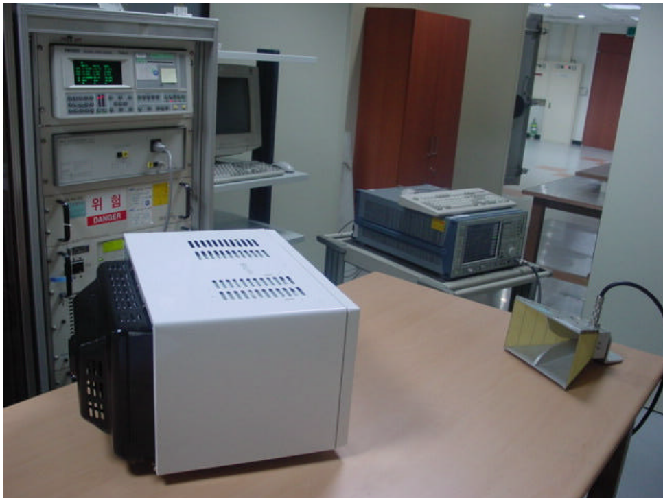
Fig. 2 Test Setup for Operating Frequency Measurements
