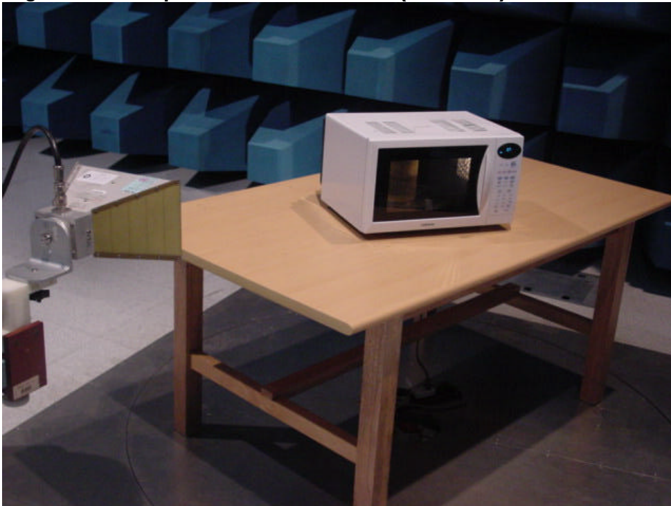
Fig. 4 Test Setup for Radiated Emission(1 - 25GHz)
