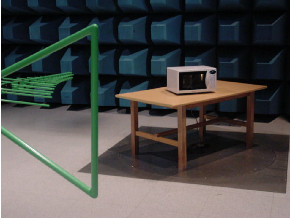
Fig. 3 Test Setup for Radiated Emission(30 - 1000MHz)
