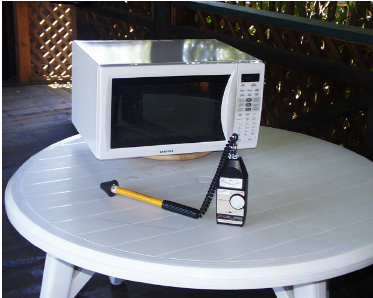
RF Hazard Test Setup
