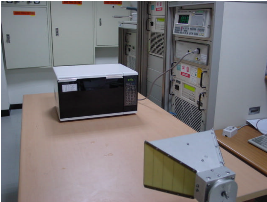
Fig. 2 Test Setup for Input power
