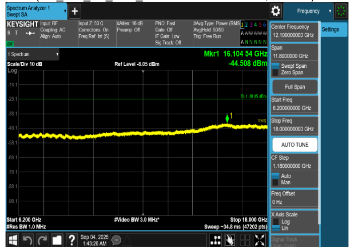
Plot 8-311. Conducted Spurious Emission Plot 6.2 GHz to 18 GHz (NR_n25_1C_10M_64QAM - Low Channel, Port 28)
