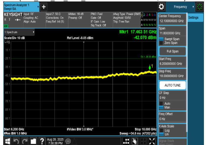
Plot 8-275. Conducted Spurious Emission Plot 6.2 GHz to 18 GHz
