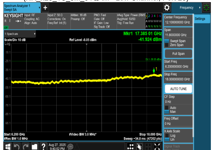
Plot 8-302. Conducted Spurious Emission Plot 6.2 GHz to 18 GHz (NR_n25_1C_5M_64QAM - Low Channel, Port 26)
