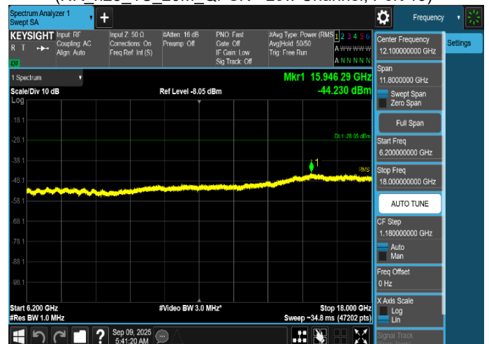
Plot 8-329. Conducted Spurious Emission Plot 6.2 GHz to 18 GHz (NR_n25_1C_20M_QPSK - Low Channel, Port 19)
