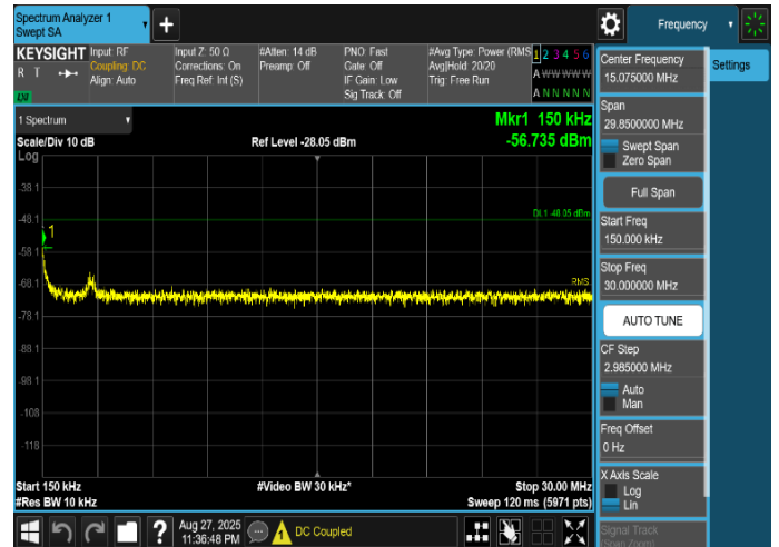
Plot 8-278. Conducted Spurious Emission Plot 150 kHz to 30 MHz
