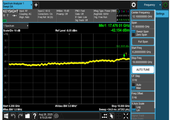
Plot 8-266. Conducted Spurious Emission Plot 6.2 GHz to 18 GHz
