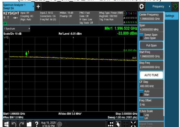
Plot 8-264. Conducted Spurious Emission Plot 1.996 GHz to 2 GHz
