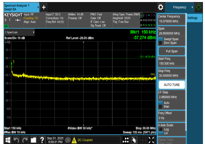
Plot 8-305. Conducted Spurious Emission Plot 150 kHz to 30 MHz (NR_n25_1C_10M_64QAM - Low Channel, Port 28)
