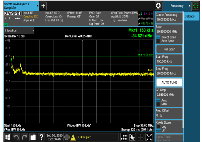
Plot 8-424. Conducted Spurious Emission Plot 150 kHz to 30 MHz
