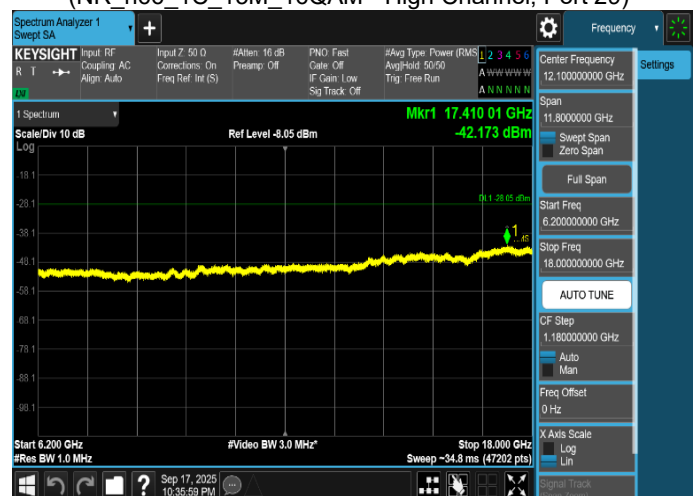
Plot 8-466. Conducted Spurious Emission Plot 6.2 GHz to 18 GHz
