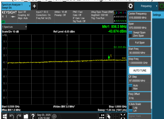
Plot 8-416. Conducted Spurious Emission Plot 30 MHz to 1 GHz
