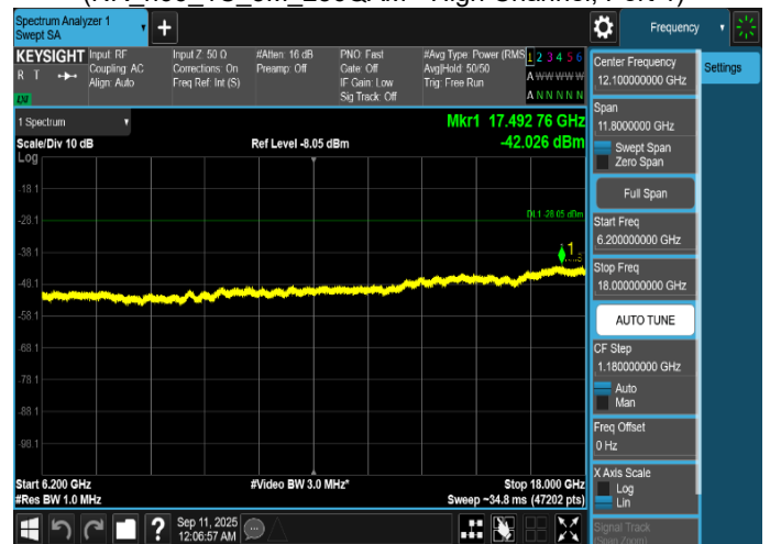
Plot 8-448. Conducted Spurious Emission Plot 6.2 GHz to 18 GHz (NR_n66_1C_5M_256QAM - High Channel, Port 4)
