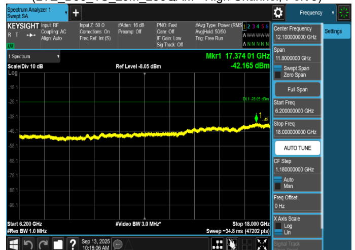
Plot 8-439. Conducted Spurious Emission Plot 6.2 GHz to 18 GHz
