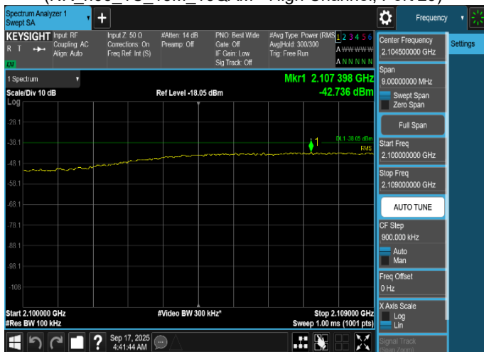
Plot 8-463. Conducted Spurious Emission Plot 2.1 GHz to 2.109 GHz
