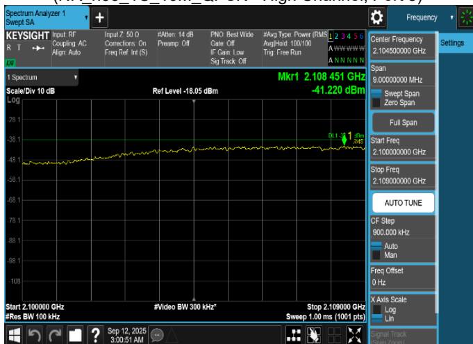
Plot 8-454. Conducted Spurious Emission Plot 2.1 GHz to 2.109 GHz (NR_n66_1C_10M_QPSK - High Channel, Port 5)
