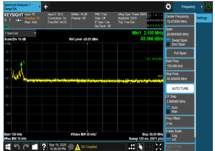
Plot 8-469. Conducted Spurious Emission Plot 150 kHz to 30 MHz
