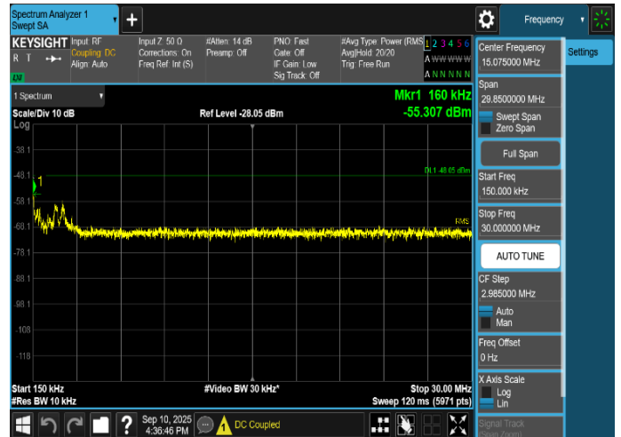
Plot 8-442. Conducted Spurious Emission Plot 150 kHz to 30 MHz
