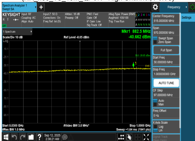
Plot 8-452. Conducted Spurious Emission Plot 30 MHz to 1 GHz (NR_n66_1C_10M_QPSK - High Channel, Port 5)
