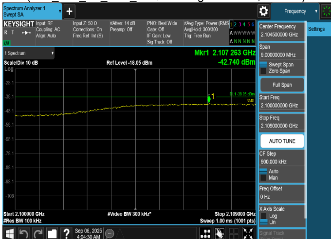
Plot 8-427. Conducted Spurious Emission Plot 2.1 GHz to 2.109 GHz
