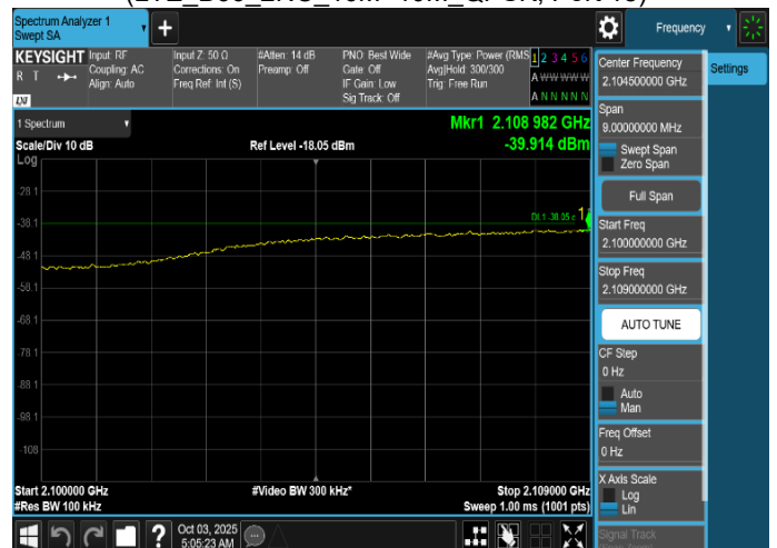
Plot 8-537. Conducted Spurious Emission Plot 2.1 GHz to 2.109 GHz (LTE_B66_2NC_10M+10M_QPSK, Port 18)
