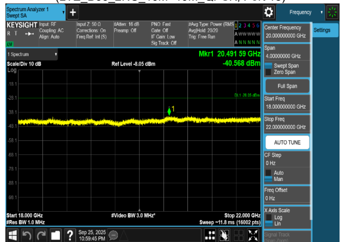
Plot 8-541. Conducted Spurious Emission Plot 18 GHz to 22 GHz (LTE_B66_2NC_10M+10M_QPSK, Port 18)
