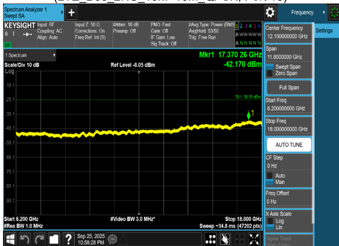
Plot 8-540. Conducted Spurious Emission Plot 6.2 GHz to 18 GHz (LTE_B66_2NC_10M+10M_QPSK, Port 18)
