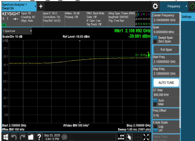
Plot 8-490. Conducted Spurious Emission Plot 2.1 GHz to 2.109 GHz (NR_n66_1C_30M_16QAM - Low Channel, Port 18)
