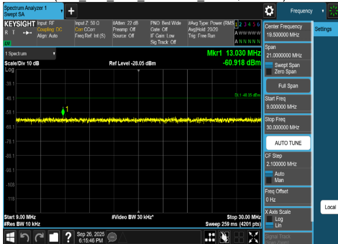
Plot 8-534. Conducted Spurious Emission Plot 9 MHz to 30 MHz (LTE_B66_2NC_10M+10M_QPSK, Port 18)
