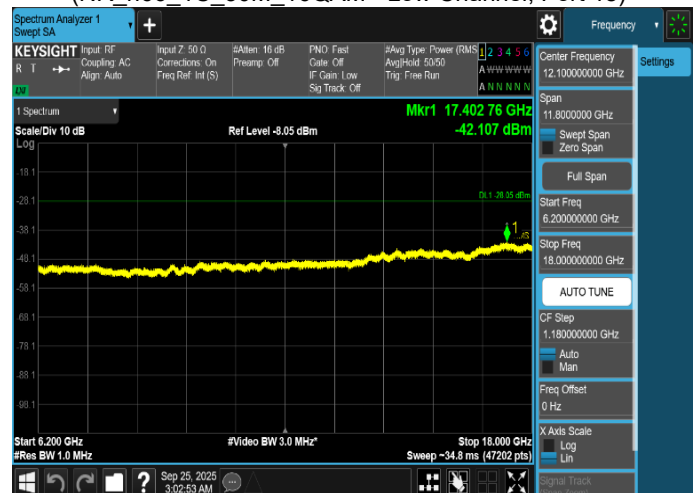
Plot 8-493. Conducted Spurious Emission Plot 6.2 GHz to 18 GHz (NR_n66_1C_30M_16QAM - Low Channel, Port 18)
