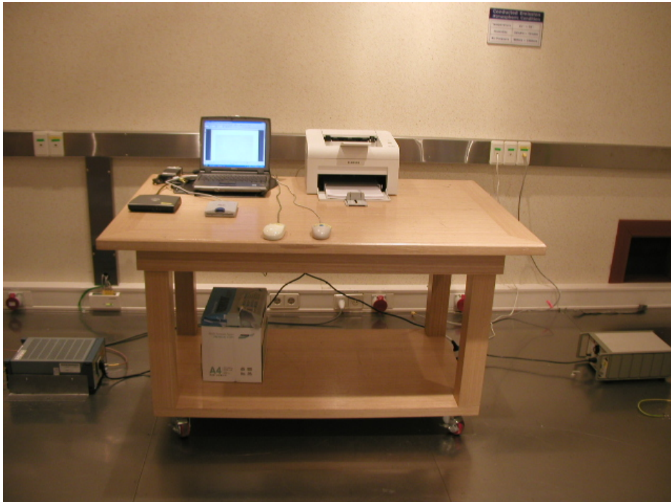
Picture 1. Conducted Emission (Front)
