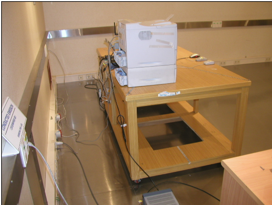
Picture 2- Conducted Emission (Rear)
