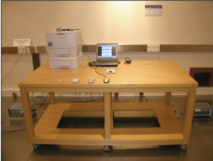
Picture 1- Conducted Emission (Front)
