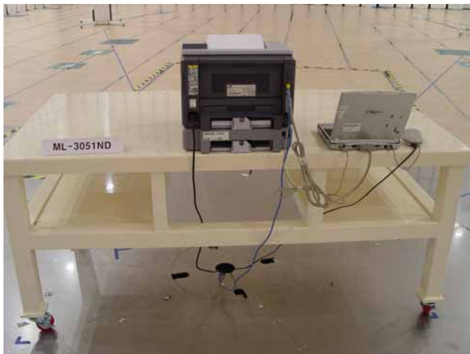
Picture 4. Radiated emission (Rear)
