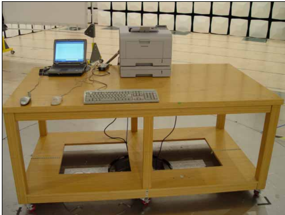
Picture 3. Radiated emission (Front)
