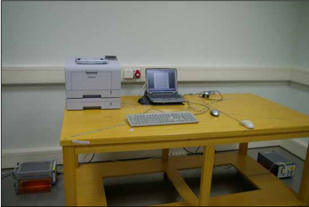
Picture 1. Conducted Emission (Front)
