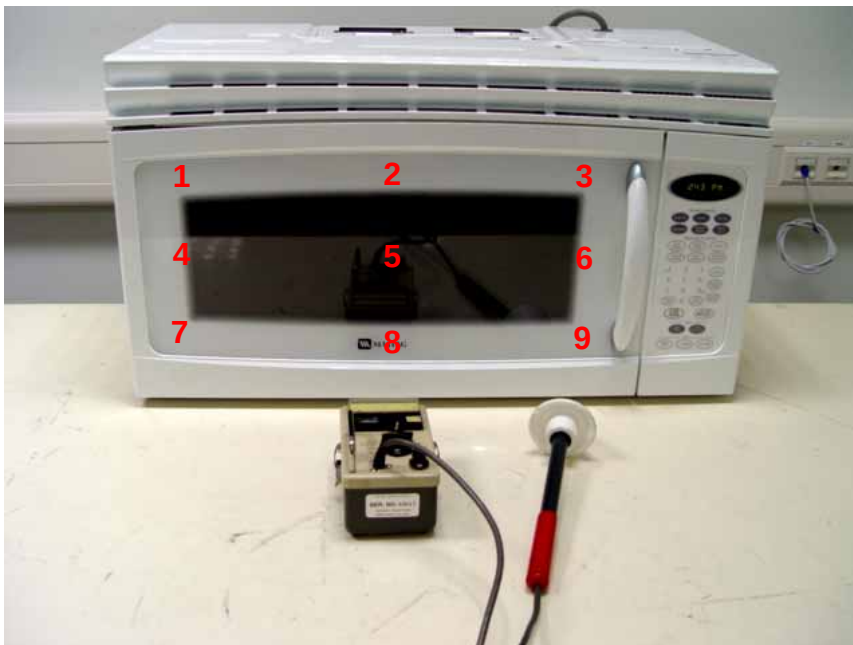
Fig. 1 Test Setup for Radiation Hazard Measurement
