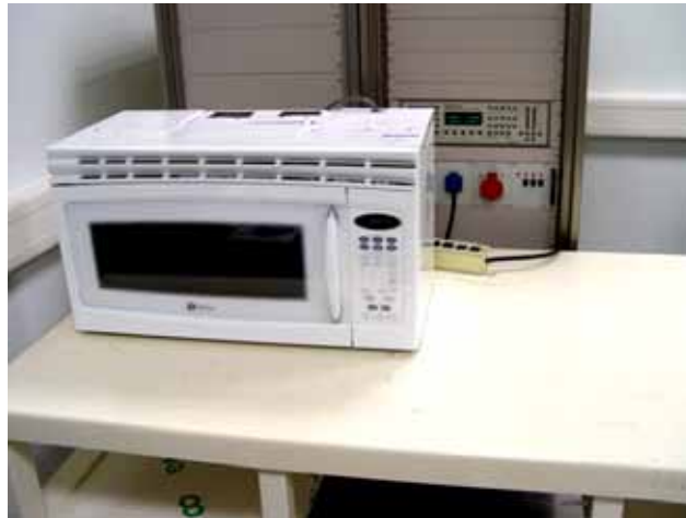
Fig.3 Test Setup for RF output power
