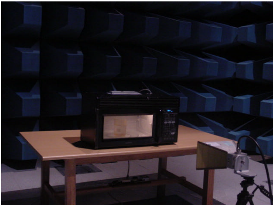
Fig. 4 Test Setup for Radiated Emission(1 - 25GHz)
