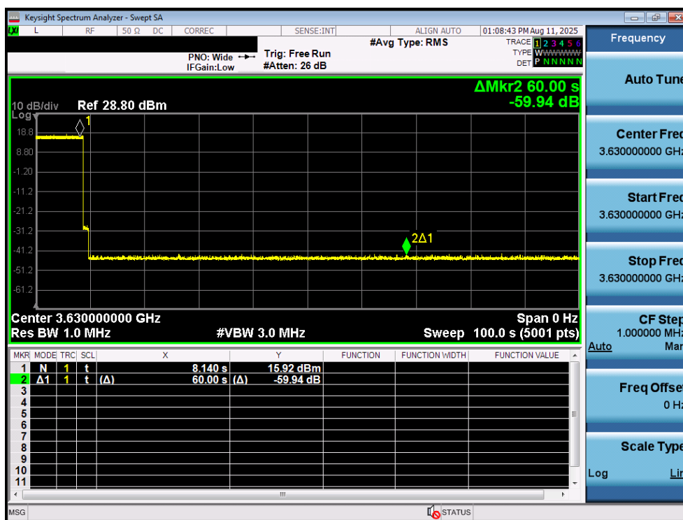
Plot 18. Conducted Measurement – RF transmission stops within 60s of SAS RLQ response (Marker 1) (WINNF.FT.C.RLQ.1)
