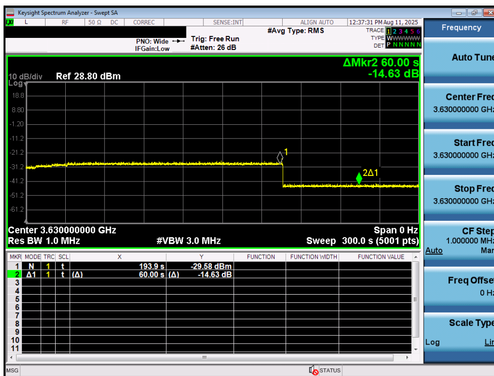
Plot 17. Conducted Measurement - RF transmission stops within 60s of SAS heartbeat response (Marker 1) (WINNF.FT.C.HBT.10)
