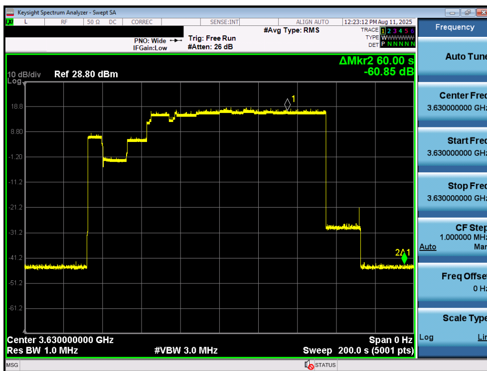
Plot 15. Conducted Measurement – RF transmission stops within 60s of SAS heartbeat response (Marker 1) (WINNF.FT.C.HBT.7)
