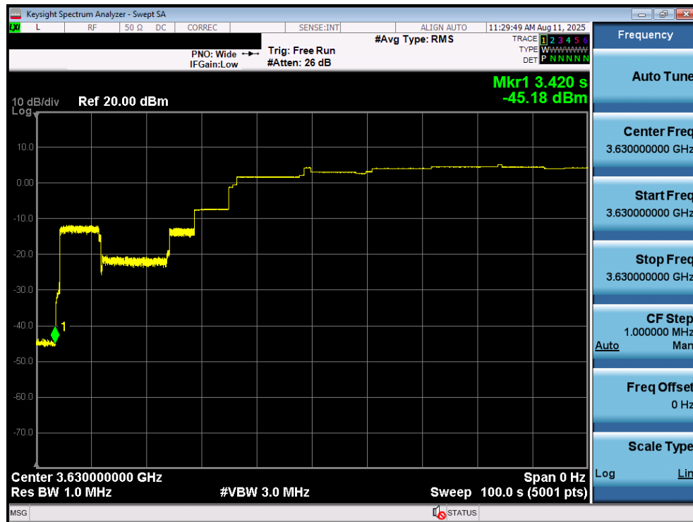
Plot 10. Conducted Measurement - RF transmission after SAS heartbeat response noted by marker 1 (WINNF.FT.C.HBT.1)
