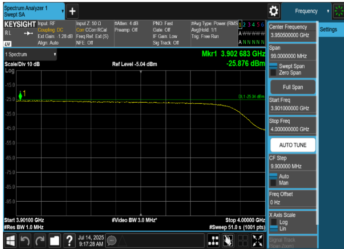
Plot 8-126. Conducted Spurious Emission Plot 3.901 GHz to 4 GHz (n48_4C_20M+20M+20M+20M+n77_2C_100M+100M QPSK, Port 13)
