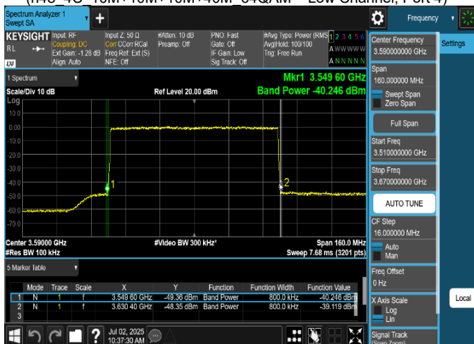
Plot 8-55. Channel Edge Emission Plot (Resolution bandwidth 1% of fundamental for measurements within 1 MHz immediately outside band power) (n48_1C_80M_256QAM – Low Channel, Port 10)
