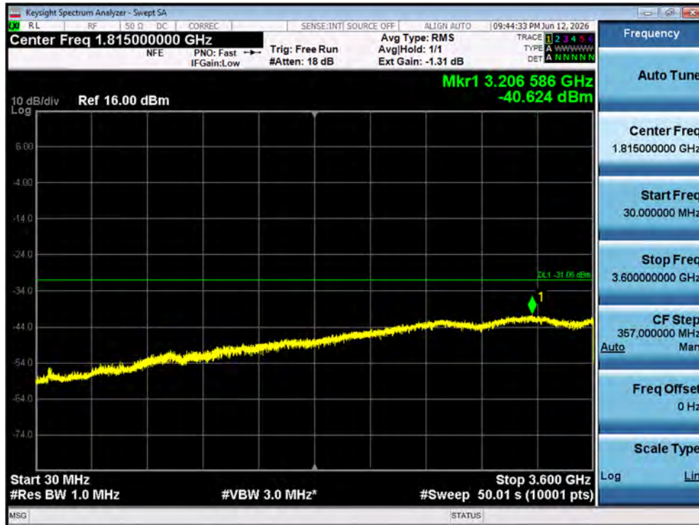
Port 27 / (64 Port) 5G NR n77 20 MHz [1 Carrier] / 30 MHz ~ Low Edge - 100 MHz / 16QAM / Low
