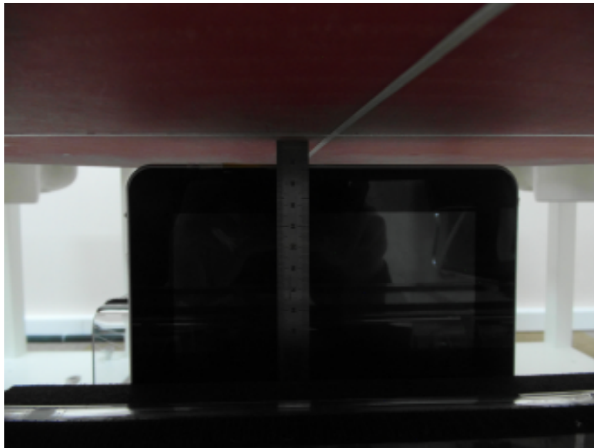
f) Right Edge Separation distance 11.0[mm]
