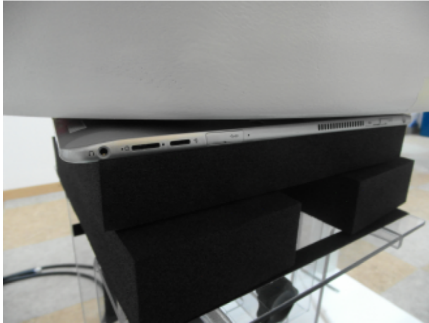
b) Rear Separation distance 14.0[mm]
