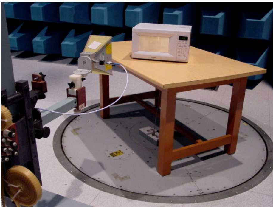
Fig. 9 Radiated Emission setup(1 - 25GHz)
