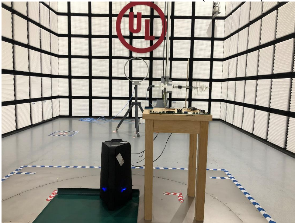
RADIATED RF MEASUREMENT SETUP (Below 30MHz)
