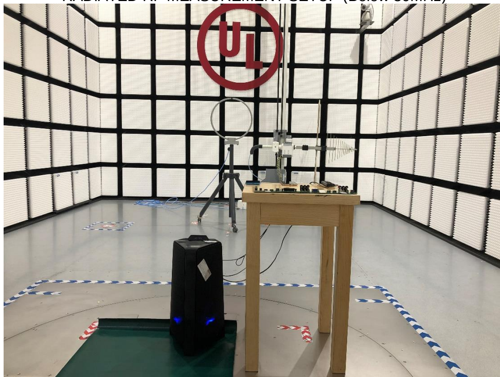
RADIATED RF MEASUREMENT SETUP (Below 30MHz)
