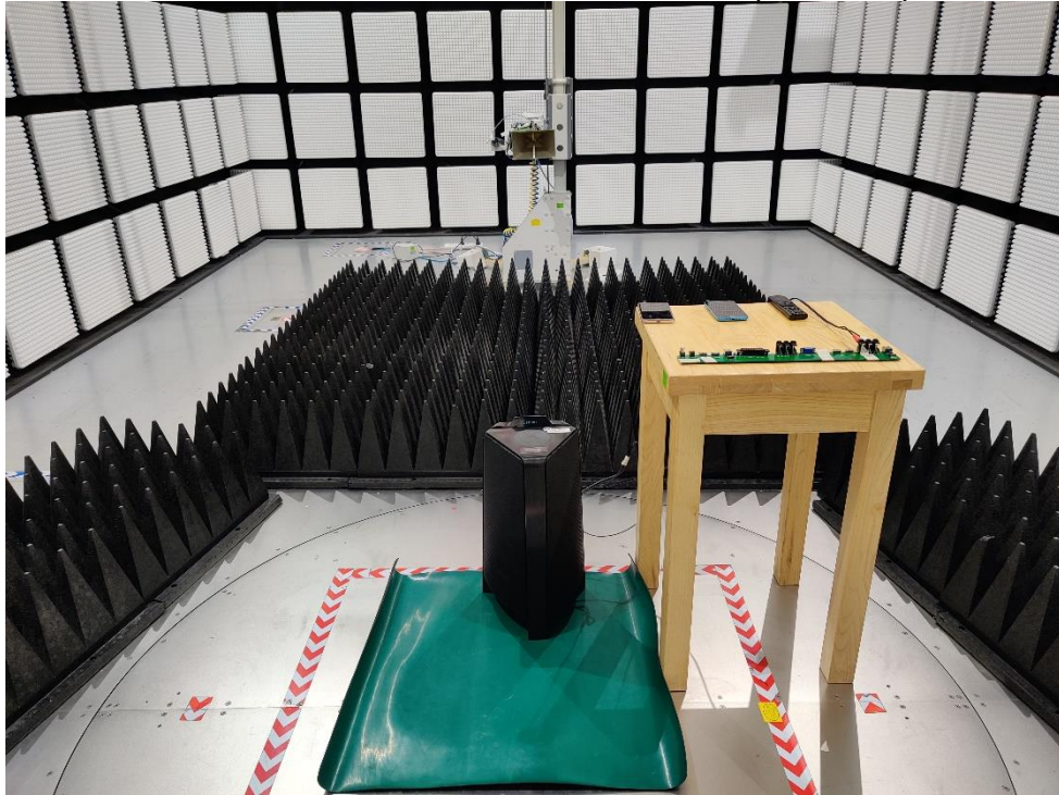
RADIATED RF MEASUREMENT SETUP (Above 1G)
