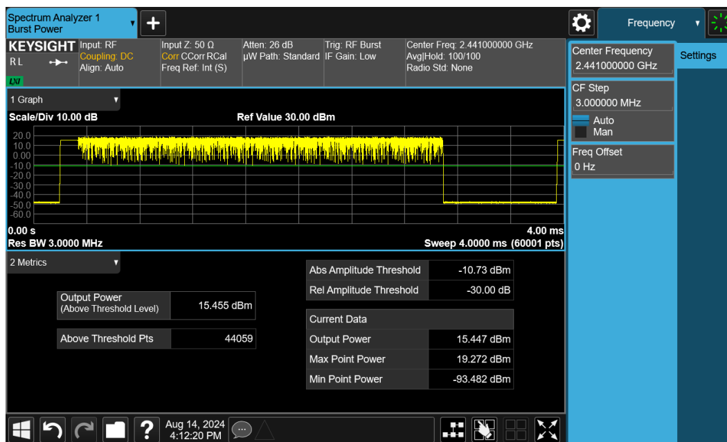
Plot 7-53. Average Conducted Power (3Mbps – Ch. 39) – Ant 1
