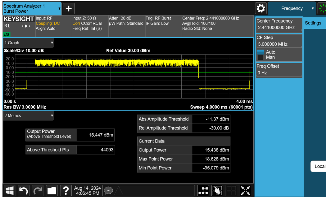
Plot 7-50. Average Conducted Power (2Mbps – Ch. 39) – Ant 1
