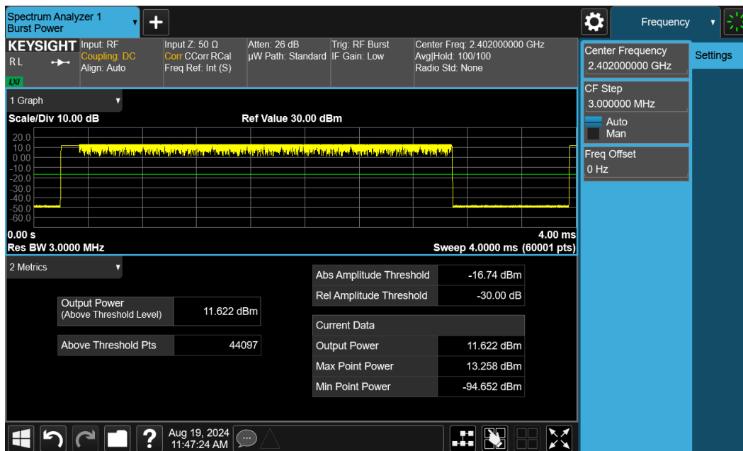
Plot 7-85. Average Conducted Power (2Mbps – Ch. 0) – Dual Ant 1
