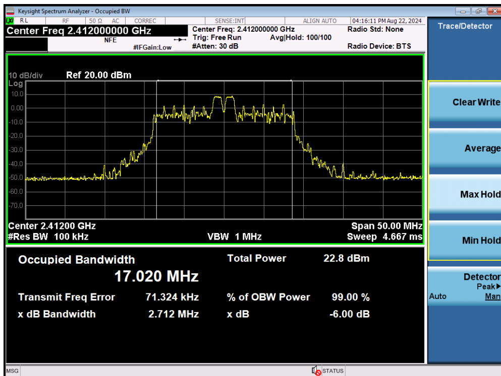
Plot 7-13. 6dB Bandwidth Plot MIMO ANT2 (802.11ax OFDMA – 26Tones – Ch. 1)
