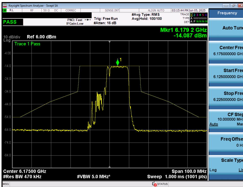
Plot 7-62. In Band Emissions Plot MIMO ANT1 (20MHz 802.11be (106+26 Tones) (UNII Band 5) – Ch. 45) - VLP
