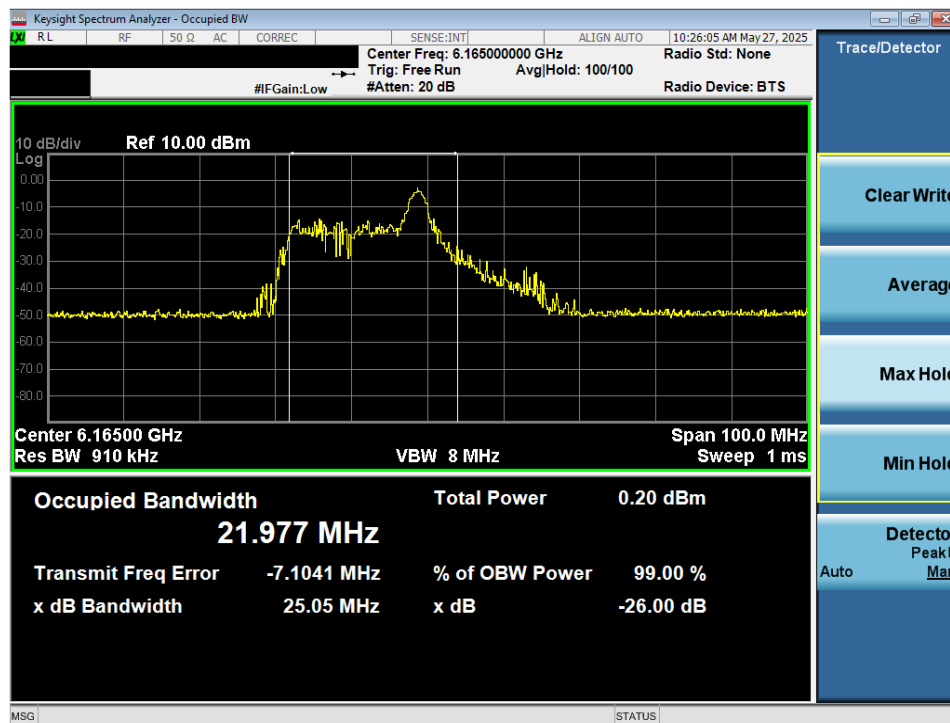
Plot 7-16. 26dB Bandwidth Plot MIMO ANT2 (40MHz 802.11ax/be (26 Tones) (UNII Band 5) – Ch. 43) - VLP
