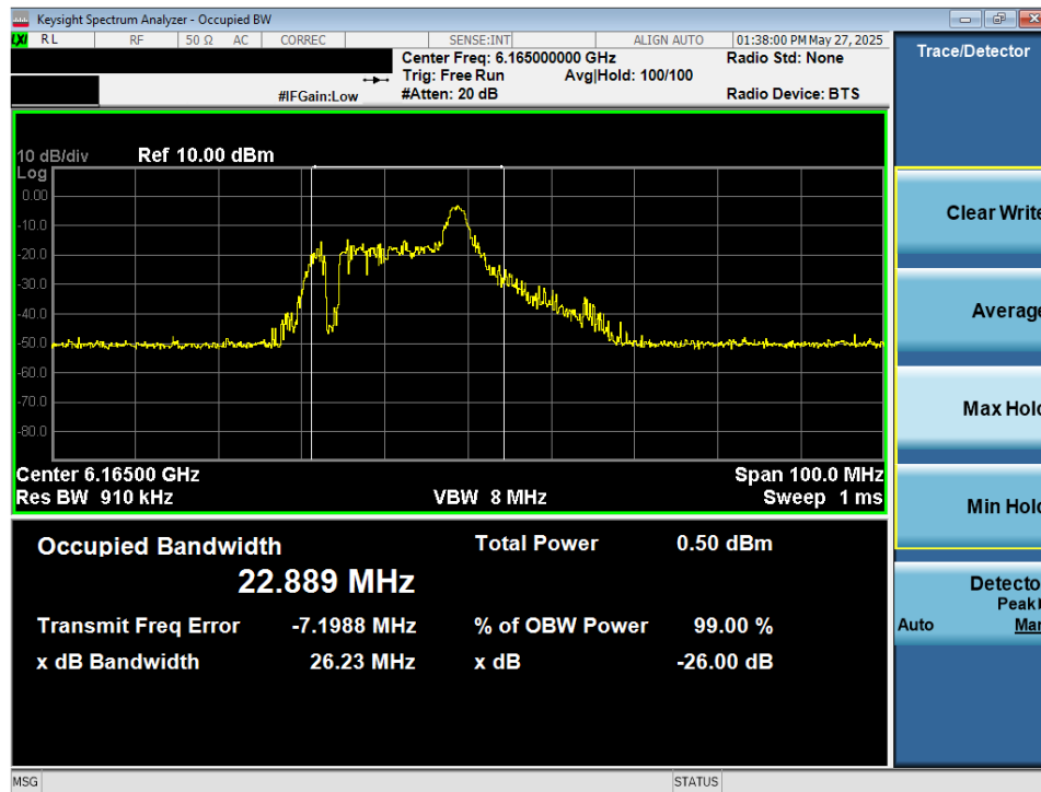
Plot 7-2. 26dB Bandwidth Plot MIMO ANT1 (40MHz 802.11ax/be (26 Tones) (UNII Band 5) – Ch. 43) - VLP
