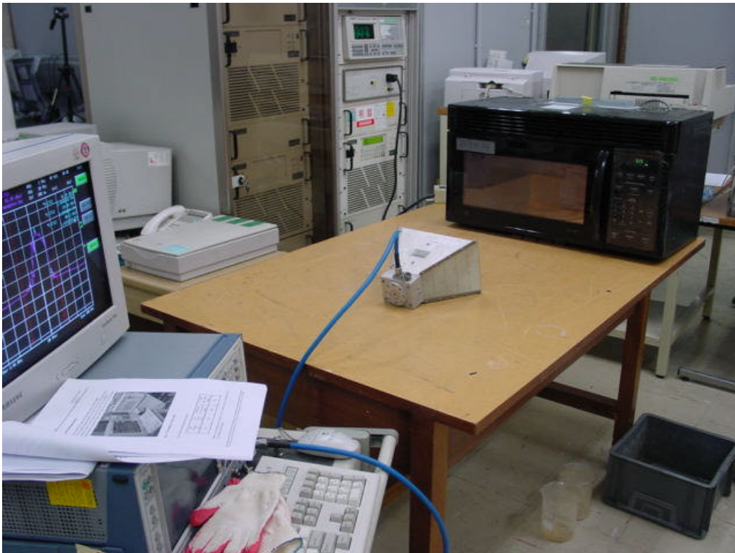
Fig. 5 Test Setup for Operating Frequency Measurements
