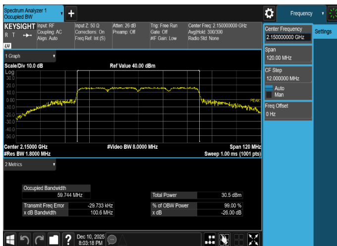
Plot 8-41. Occupied Bandwidth Plot (LTE_B66_4C_15M+15M+15M+15M_QPSK - High Channel, Port 0)
