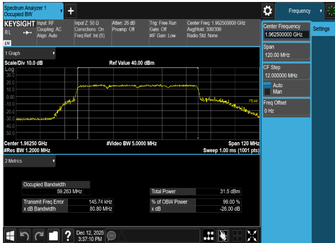
Plot 8-25. Occupied Bandwidth Plot (NR_n25_4C_15M+15M+15M+15M_QPSK - Mid Channel, Port 2)
