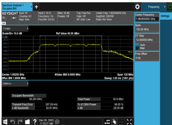
Plot 8-11. Occupied Bandwidth Plot (LTE_B25_4C_15M+15M+15M+15M_QPSK - Mid Channel, Port 2)
