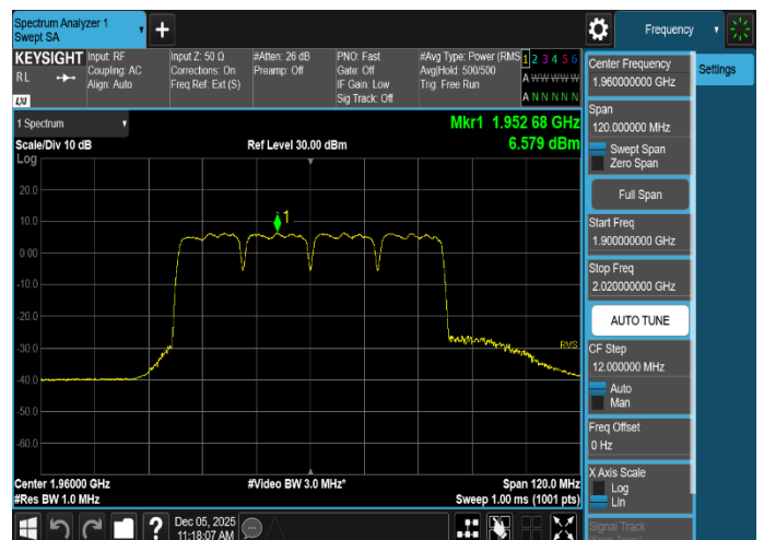
Plot 8-80. Equivalent Isotropically Radiated Power Plot (LTE_B25_4C_15M+15M+15M+15M_16QAM - Low Channel, Port 2)
