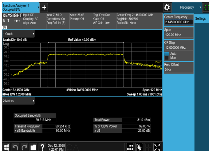
Plot 8-57. Occupied Bandwidth Plot (NR_n66_4C_15M+15M+15M_QPSK - Mid Channel, Port 1)
