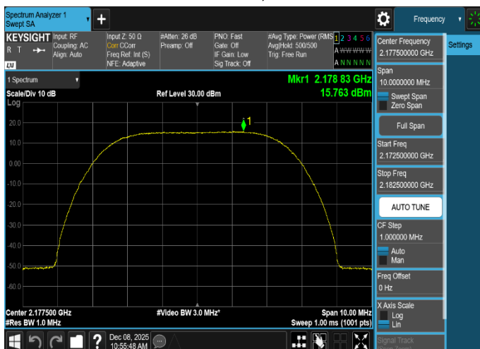
Plot 8-90. Equivalent Isotropically Radiated Power Plot (LTE_B66_1C_5M_16QAM - High Channel, Port 1)
