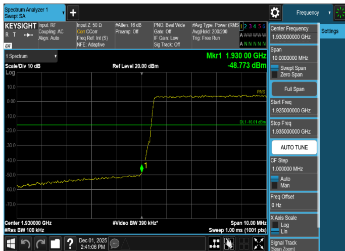
Plot 8-149. Band Edge Emission Summary Data Plot (LTE_B25_1C_10M_256QAM - Low Edge, Port 2)
