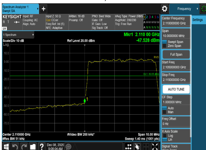
Plot 8-159. Band Edge Emission Summary Data Plot (LTE_B66_1C_5M_16QAM - Low Edge, Port 0)
