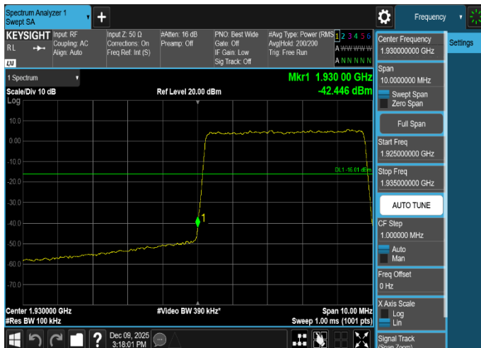
Plot 8-157. Band Edge Emission Summary Data Plot (MSR_B/n25_2NC_LTE_5M+NR_5M_QPSK - Low Edge, Port 2)
