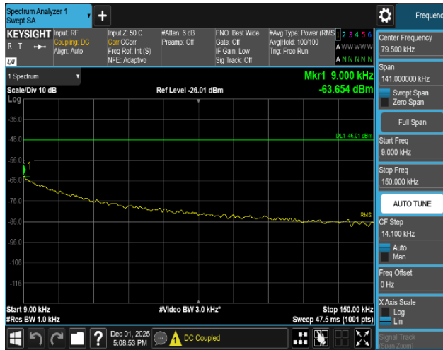
Plot 8-173. Conducted Spurious Emission Plot 9 kHz to 150 kHz
