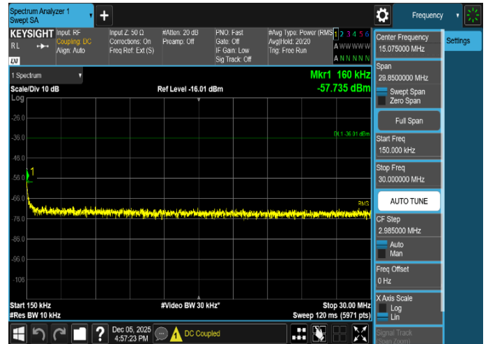
Plot 8-201. Conducted Spurious Emission Plot 150 kHz to 30 MHz
