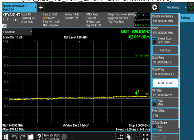
Plot 8-193. Conducted Spurious Emission Plot 30 MHz to 1 GHz
