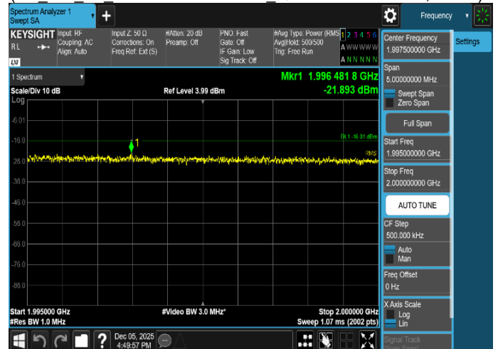
Plot 8-205. Conducted Spurious Emission Plot 1.995 GHz to 2 GHz
