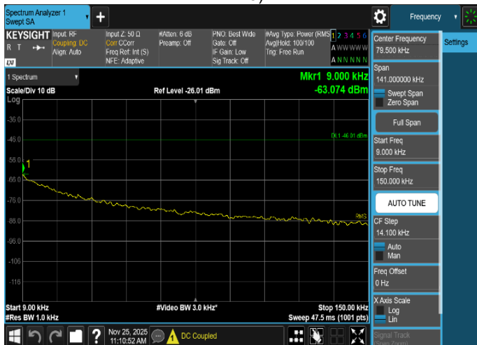
Plot 8-191. Conducted Spurious Emission Plot 9 kHz to 150 kHz
