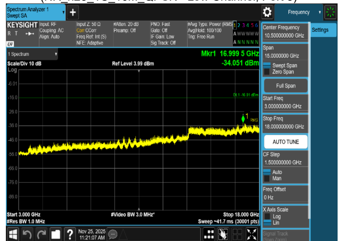
Plot 8-198. Conducted Spurious Emission Plot 3 GHz to 18 GHz (NR_n25_1C_10M_QPSK - Low Channel, Port 3)
