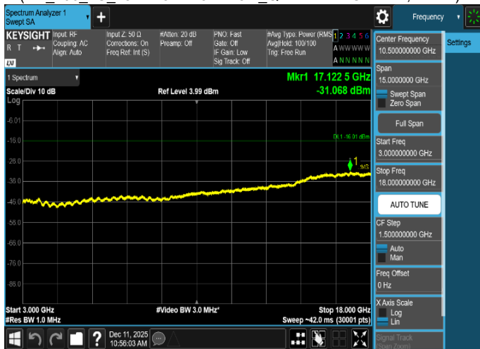
Plot 8-248. Conducted Spurious Emission Plot 3 GHz to 18 GHz
