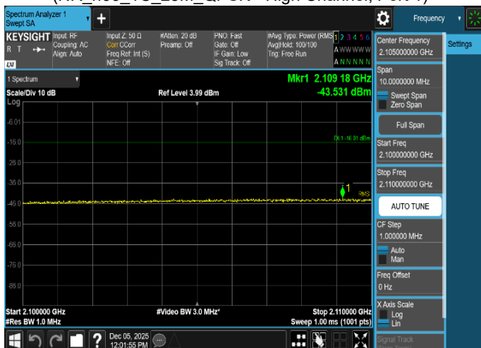
Plot 8-238. Conducted Spurious Emission Plot 2.1 GHz to 2.11 GHz
