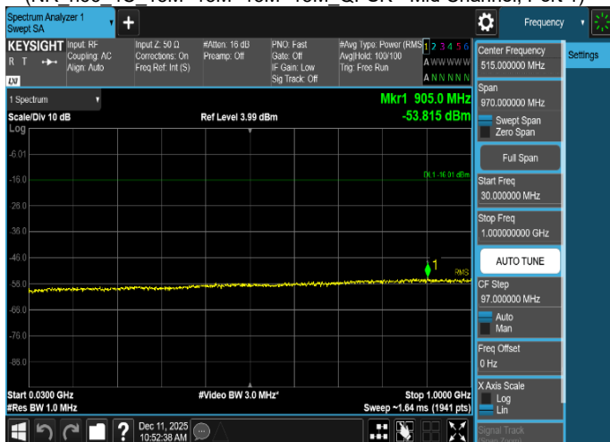
Plot 8-244. Conducted Spurious Emission Plot 30 MHz to 1 GHz
