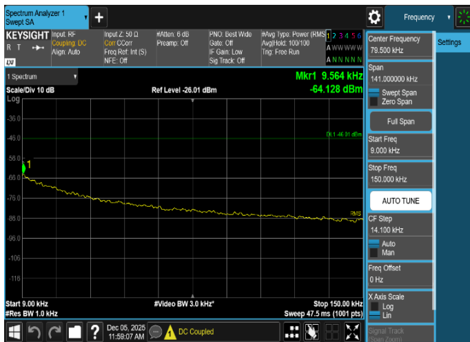
Plot 8-234. Conducted Spurious Emission Plot 9 kHz to 150 kHz
