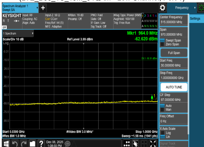
Plot 8-220. Conducted Spurious Emission Plot 30 MHz to 1 GHz
