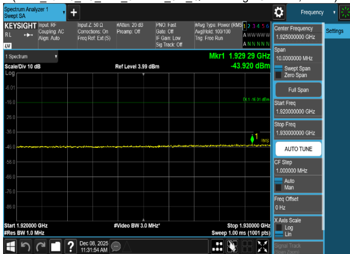
Plot 8-213. Conducted Spurious Emission Plot 1.92 GHz to 1.93 GHz (MSR_B/n25_2C_LTE_5M+NR_5M_QPSK - High Channel, Port 2)
