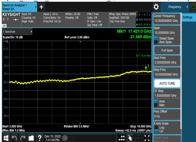
Plot 8-232. Conducted Spurious Emission Plot 3 GHz to 18 GHz
