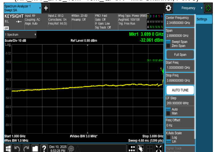
Plot 8-268. Conducted Spurious Emission Plot 1 GHz to 3.699 GHz (NR_n77_2NC_40M+40M_QPSK - Mid Channel, Port 5)
