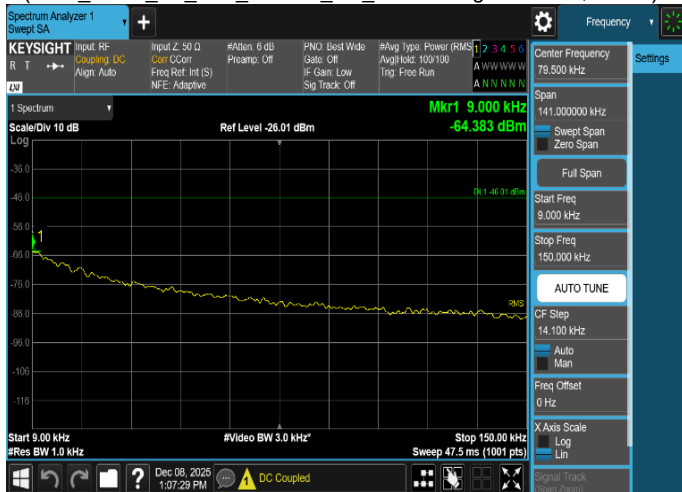
Plot 8-218. Conducted Spurious Emission Plot 9 kHz to 150 kHz
