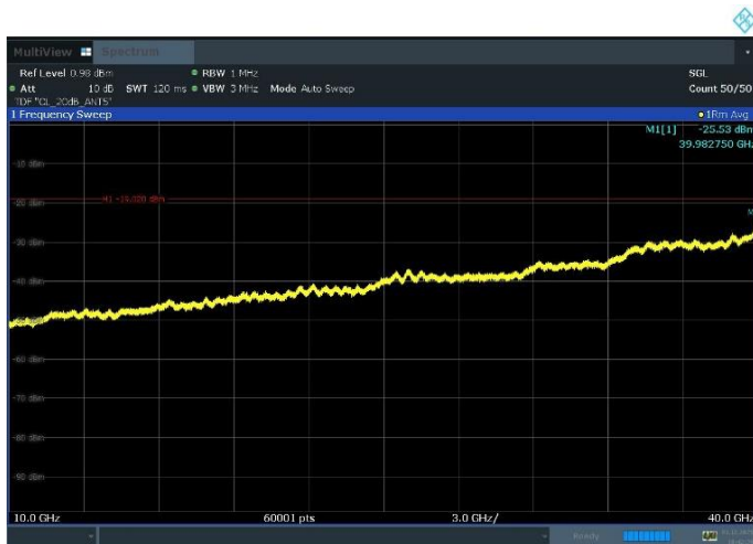
Plot 8-264. Conducted Spurious Emission Plot 10 GHz to 40 GHz (NR_n77_1C_60M_16QAM - High Channel, Port 5)
