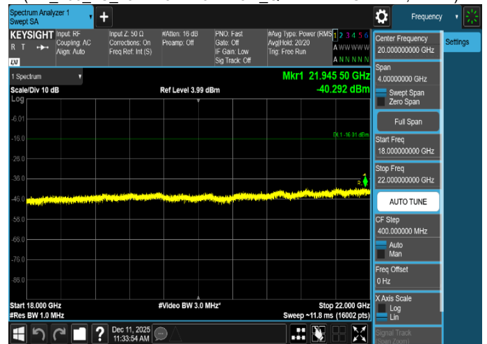
Plot 8-249. Conducted Spurious Emission Plot 18 GHz to 22 GHz
