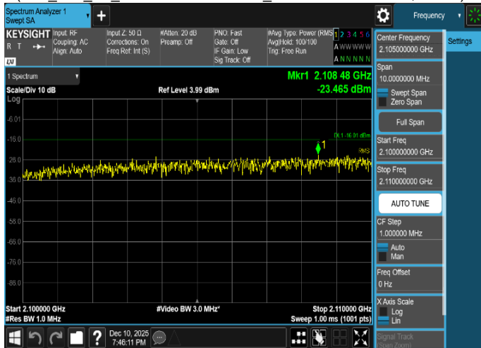
Plot 8-230. Conducted Spurious Emission Plot 2.1 GHz to 2.11 GHz
