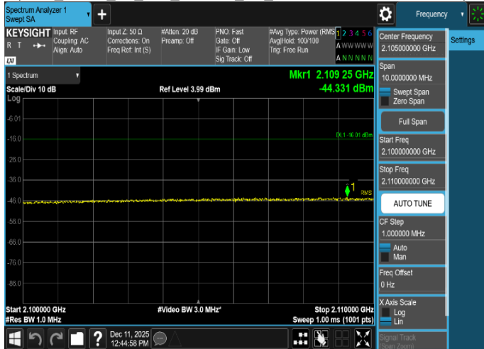
Plot 8-254. Conducted Spurious Emission Plot 2.1 GHz to 2.11 GHz
