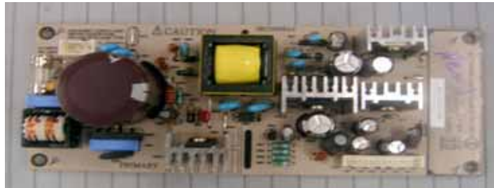
SMPS board top view
