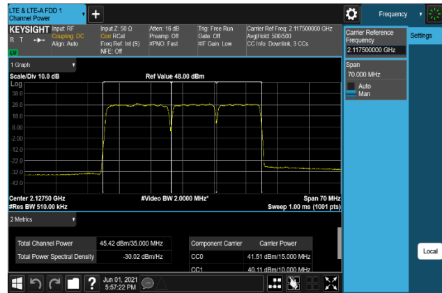
Plot 7-146. Conducted Average Output Power Plot (B66_15M+10M+10M_16QAM - Low Channel, Port 0)
