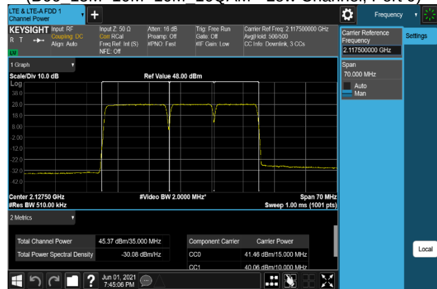
Plot 7-148. Conducted Average Output Power Plot (B66_15M+10M+10M_256QAM - Low Channel, Port 0)
