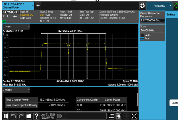
Plot 7-145. Conducted Average Output Power Plot (B66_15M+10M+10M_QPSK - Low Channel, Port 0)
