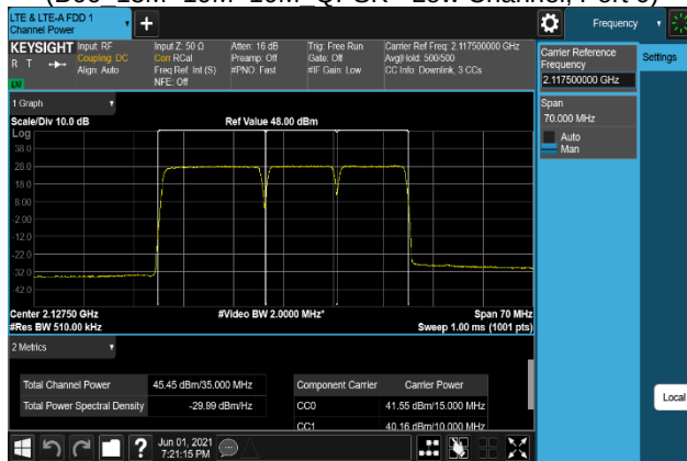
Plot 7-147. Conducted Average Output Power Plot (B66_15M+10M+10M_64QAM - Low Channel, Port 0)
