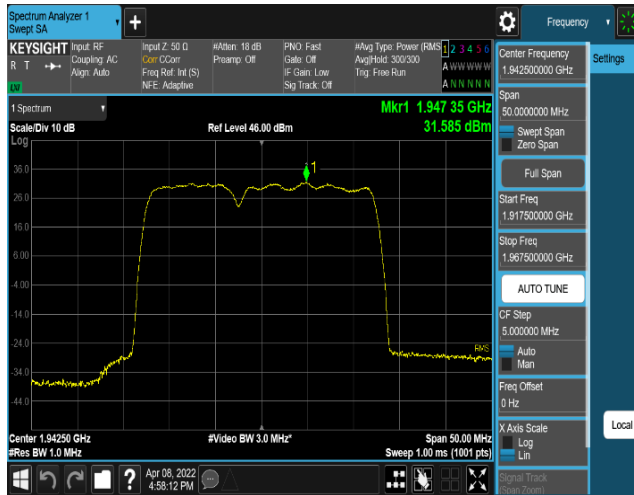
Plot 8-113. Power Spectral Density Plot (PCS DSS 2C 10M+15M 16QAM - Low Channel, Port 0)
