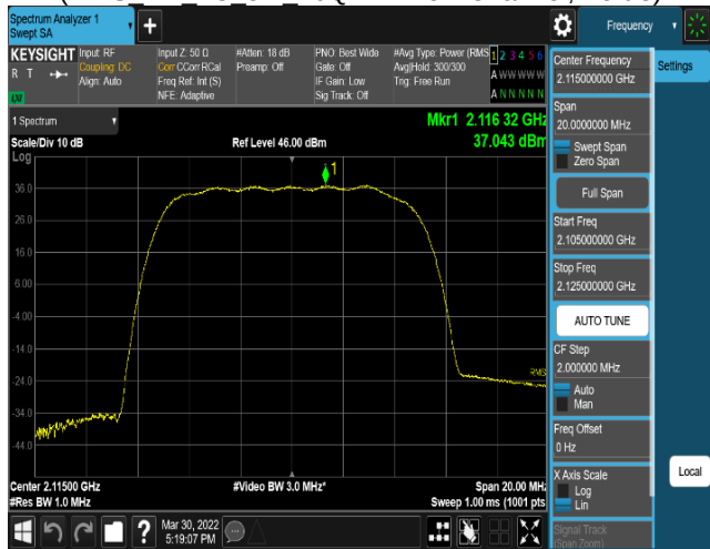
Plot 8-134. Power Spectral Density Plot (AWS NR 1C 10M 16QAM - Low Channel, Port 1)
