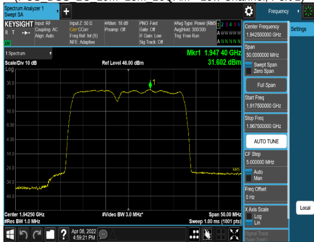
Plot 8-116. Power Spectral Density Plot (PCS DSS 2C 10M+15M 16QAM - Low Channel, Port 3)
