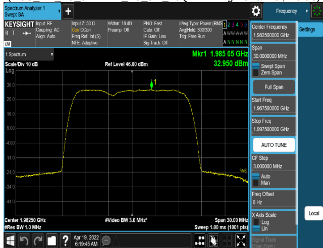
Plot 8-98. Power Spectral Density Plot (PCS DSS 1C 10M+NR 1C 5M 16QAM - High Channel, Port 1)
