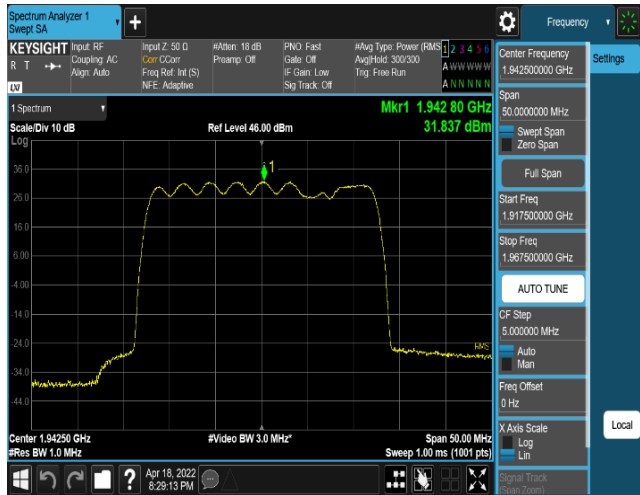
Plot 8-126. Power Spectral Density Plot (PCS_NR_1C_20M + LTE_1C_5M_16QAM - Low Channel, Port 1)
