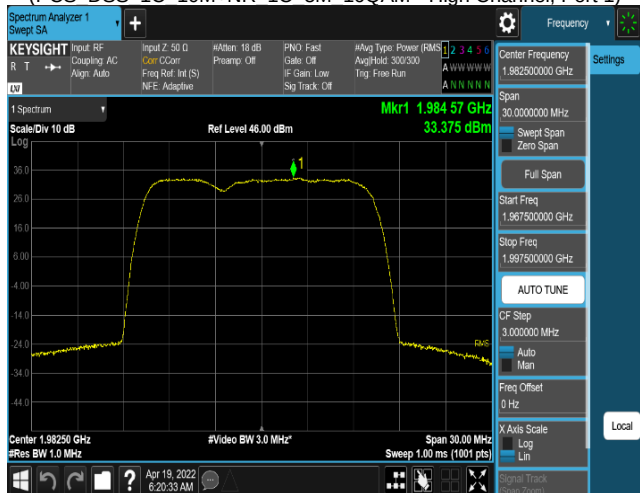
Plot 8-100. Power Spectral Density Plot (PCS DSS 1C 10M+NR 1C 5M 16QAM - High Channel, Port 3)
