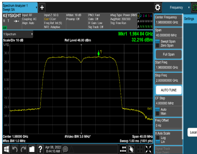
Plot 8-101. Power Spectral Density Plot (PCS DSS 2C 10M+10M 16QAM - High Channel, Port 0)
