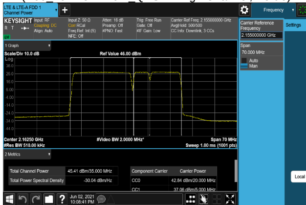
Plot 7-243. Conducted Average Output Power Plot (B66_20M+5M+10M_64QAM - High Channel, Port 0)
