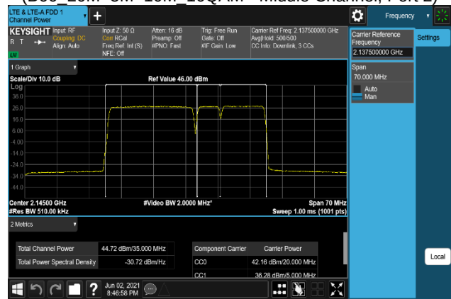
Plot 7-236. Conducted Average Output Power Plot (B66_20M+5M+10M_256QAM - Middle Channel, Port 2)
