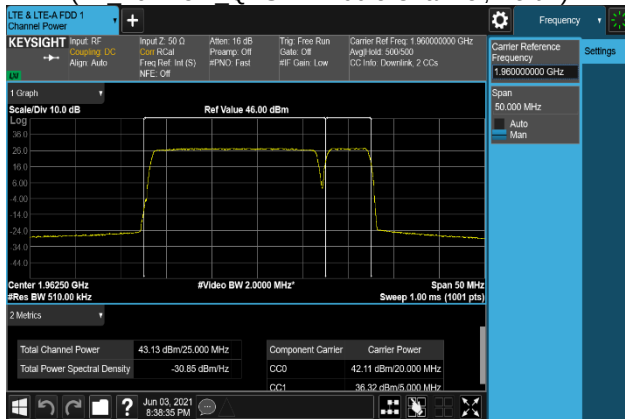
Plot 7-295. Conducted Average Output Power Plot (B2_20M+5M_64QAM - Middle Channel, Port 1)
