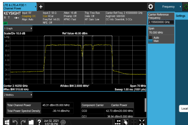
Plot 7-246. Conducted Average Output Power Plot (B66_20M+5M+10M_16QAM - High Channel, Port 1)
