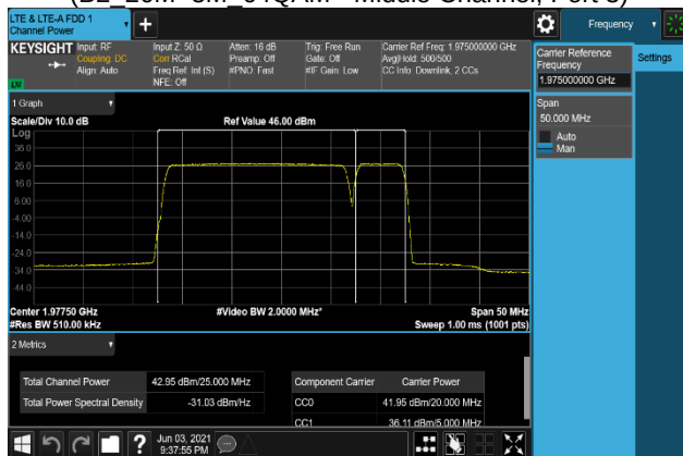
Plot 7-305. Conducted Average Output Power Plot (B2_20M+5M_QPSK - High Channel, Port 0)
