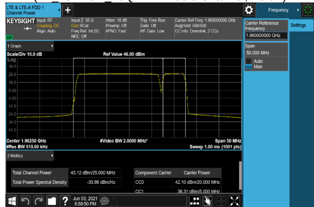
Plot 7-296. Conducted Average Output Power Plot (B2_20M+5M_256QAM - Middle Channel, Port 1)
