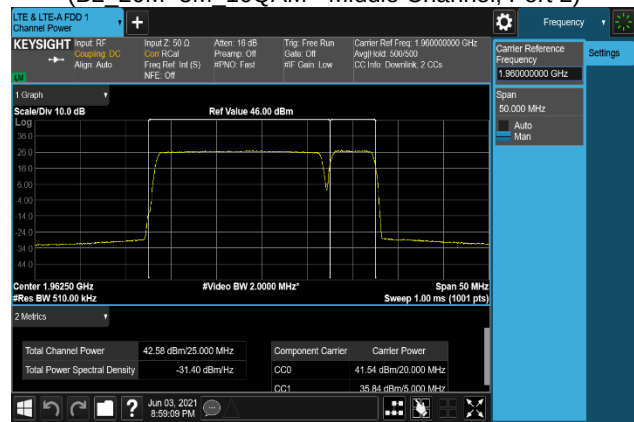
Plot 7-300. Conducted Average Output Power Plot (B2_20M+5M_256QAM - Middle Channel, Port 2)
