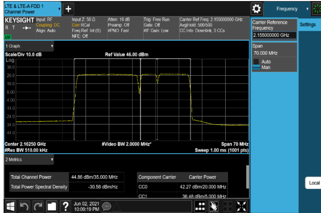
Plot 7-251. Conducted Average Output Power Plot (B66_20M+5M+10M_64QAM - High Channel, Port 2)
