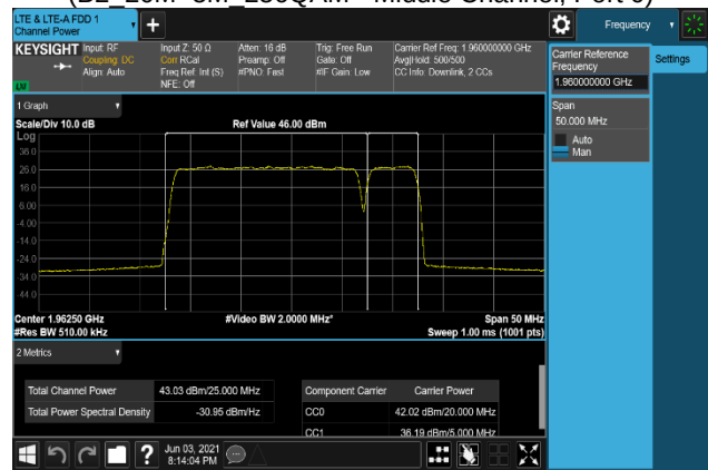
Plot 7-294. Conducted Average Output Power Plot (B2_20M+5M_16QAM - Middle Channel, Port 1)
