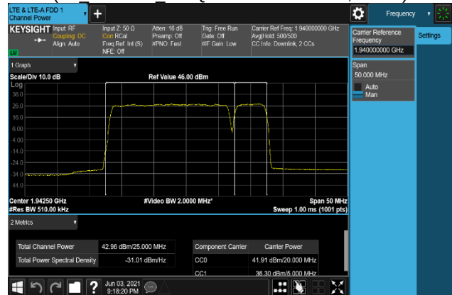
Plot 7-278. Conducted Average Output Power Plot (B2_20M+5M_16QAM - Low Channel, Port 1)
