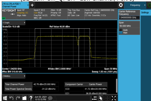
Plot 7-275. Conducted Average Output Power Plot (B2_20M+5M_64QAM - Low Channel, Port 0)
