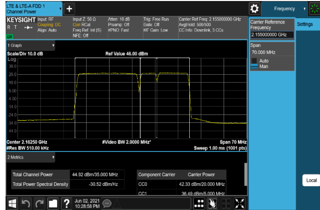
Plot 7-252. Conducted Average Output Power Plot (B66_20M+5M+10M_256QAM - High Channel, Port 2)
