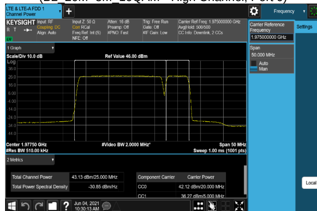
Plot 7-308. Conducted Average Output Power Plot (B2_20M+5M_256QAM - High Channel, Port 0)
