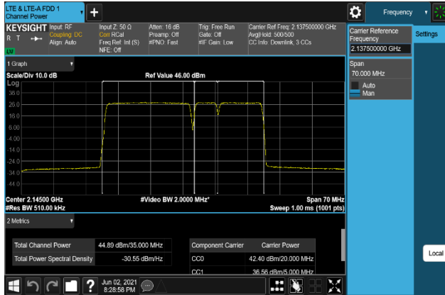
Plot 7-239. Conducted Average Output Power Plot (B66_20M+5M+10M_64QAM - Middle Channel, Port 3)
