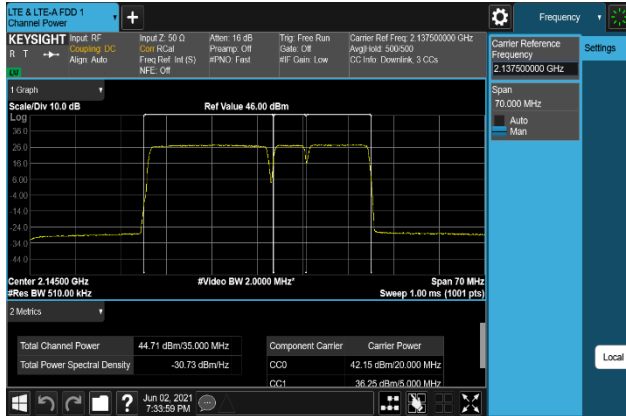
Plot 7-233. Conducted Average Output Power Plot (B66_20M+5M+10M_QPSK - Middle Channel, Port 2)
