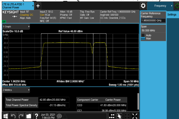
Plot 7-289. Conducted Average Output Power Plot (B2_20M+5M_QPSK - Middle Channel, Port 0)
