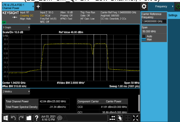
Plot 7-287. Conducted Average Output Power Plot (B2_20M+5M_64QAM - Low Channel, Port 3)
