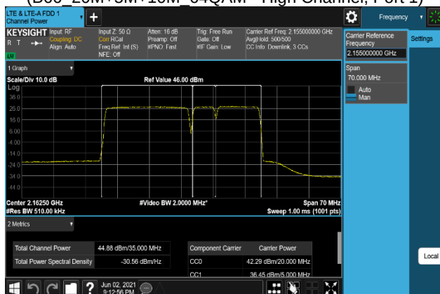
Plot 7-249. Conducted Average Output Power Plot (B66_20M+5M+10M_QPSK - High Channel, Port 2)
