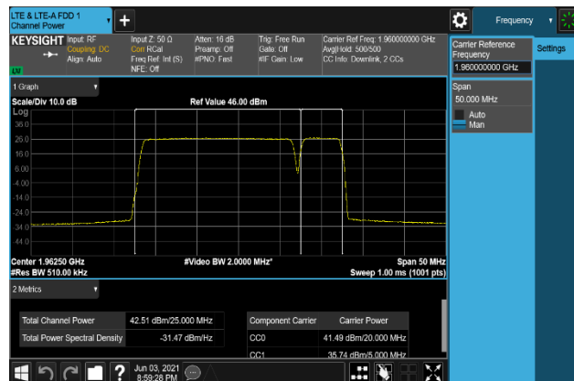
Plot 7-304. Conducted Average Output Power Plot (B2_20M+5M_256QAM - Middle Channel, Port 3)
