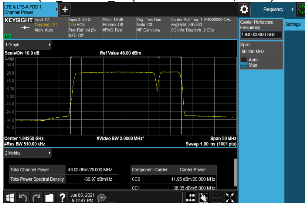
Plot 7-277. Conducted Average Output Power Plot (B2_20M+5M_QPSK - Low Channel, Port 1)
