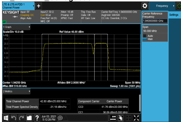
Plot 7-273. Conducted Average Output Power Plot (B2_20M+5M_QPSK - Low Channel, Port 0)
