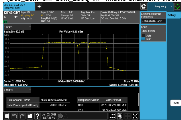
Plot 7-242. Conducted Average Output Power Plot (B66_20M+5M+10M_16QAM - High Channel, Port 0)
