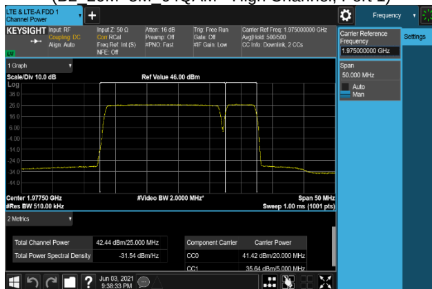
Plot 7-313. Conducted Average Output Power Plot (B2_20M+5M_QPSK - High Channel, Port 2)
