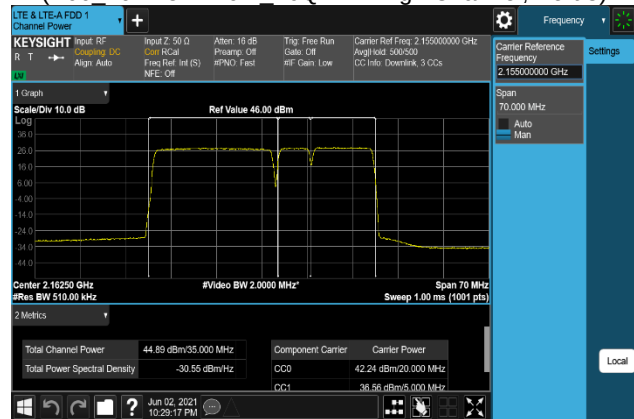
Plot 7-256. Conducted Average Output Power Plot (B66_20M+5M+10M_256QAM - High Channel, Port 3)
