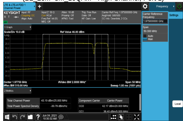
Plot 7-312. Conducted Average Output Power Plot (B2_20M+5M_256QAM - High Channel, Port 1)
