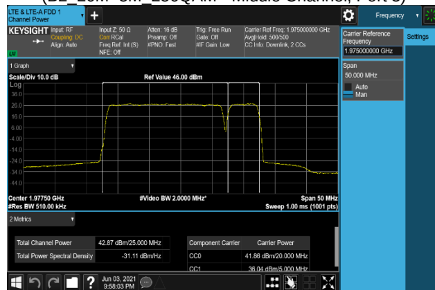
Plot 7-306. Conducted Average Output Power Plot (B2_20M+5M_16QAM - High Channel, Port 0)
