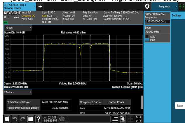
Plot 7-254. Conducted Average Output Power Plot (B66_20M+5M+10M_16QAM - High Channel, Port 3)
