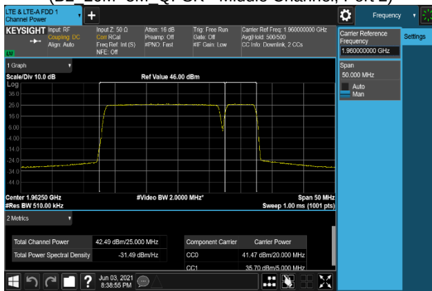
Plot 7-299. Conducted Average Output Power Plot (B2_20M+5M_64QAM - Middle Channel, Port 2)
