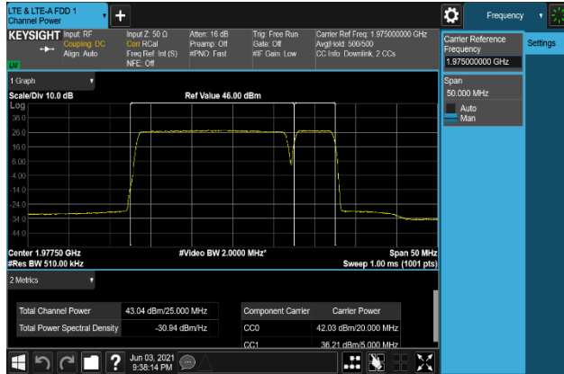
Plot 7-309. Conducted Average Output Power Plot (B2_20M+5M_QPSK - High Channel, Port 1)
