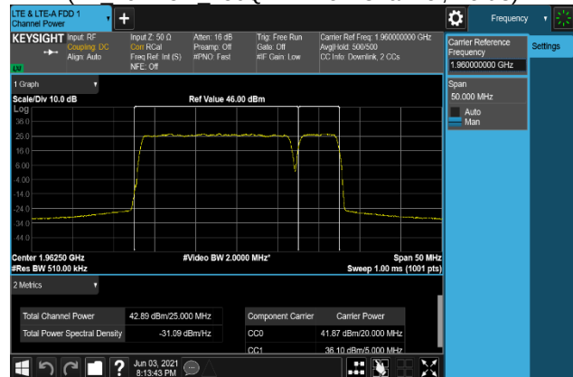
Plot 7-290. Conducted Average Output Power Plot (B2_20M+5M_16QAM - Middle Channel, Port 0)
