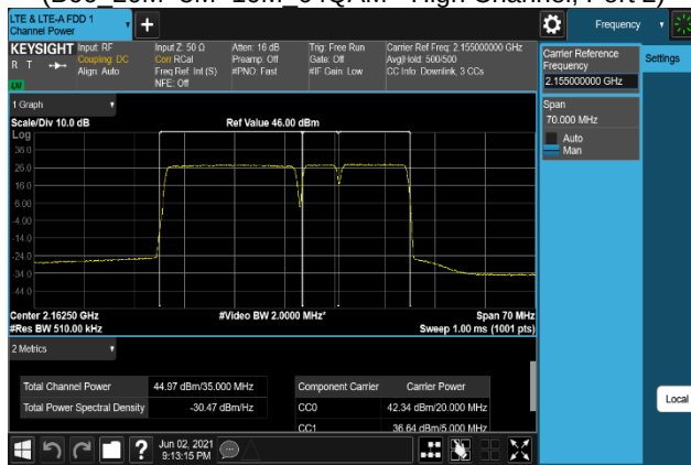
Plot 7-253. Conducted Average Output Power Plot (B66_20M+5M+10M_QPSK - High Channel, Port 3)
