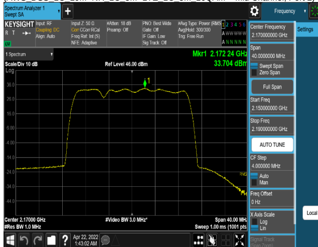
Plot 8-177. Power Spectral Density Plot (AWS_DSS_1C_15M + LTE_1C_5M_16QAM – High Channel, Port 0)
