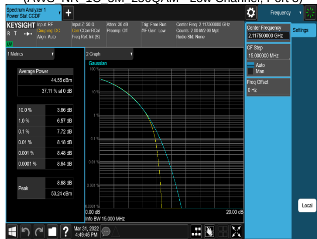
Plot 8-214. Peak To Average Power Ratio Plot (AWS_NR_1C_15M_16QAM - Low Channel, Port 3)
