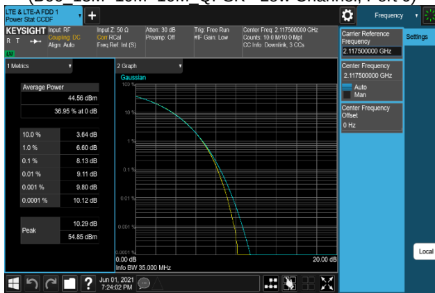
Plot 7-375. Peak To Average Power Ratio Plot (B66_15M+10M+10M_64QAM - Low Channel, Port 0)
