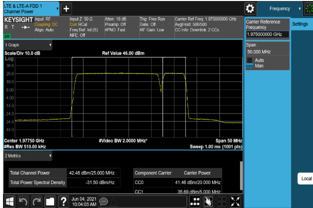
Plot 7-315. Conducted Average Output Power Plot (B2_20M+5M_64QAM - High Channel, Port 2)
