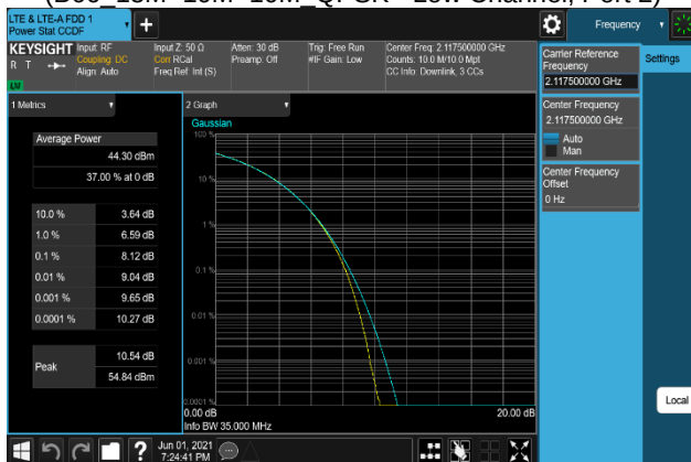
Plot 7-383. Peak To Average Power Ratio Plot (B66_15M+10M+10M_64QAM - Low Channel, Port 2)
