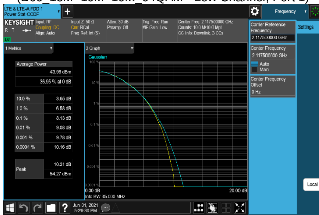
Plot 7-381. Peak To Average Power Ratio Plot (B66_15M+10M+10M_QPSK - Low Channel, Port 2)
