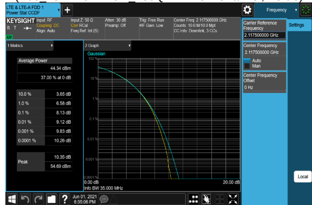
Plot 7-378. Peak To Average Power Ratio Plot (B66_15M+10M+10M_16QAM - Low Channel, Port 1)
