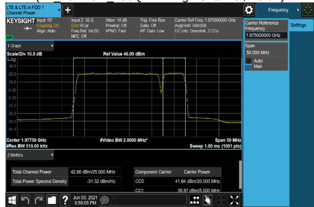
Plot 7-318. Conducted Average Output Power Plot (B2_20M+5M_16QAM - High Channel, Port 3)
