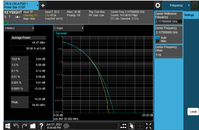
Plot 7-374. Peak To Average Power Ratio Plot (B66_15M+10M+10M_16QAM - Low Channel, Port 0)
