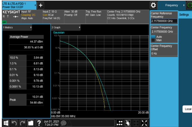
Plot 7-379. Peak To Average Power Ratio Plot (B66_15M+10M+10M_64QAM - Low Channel, Port 1)
