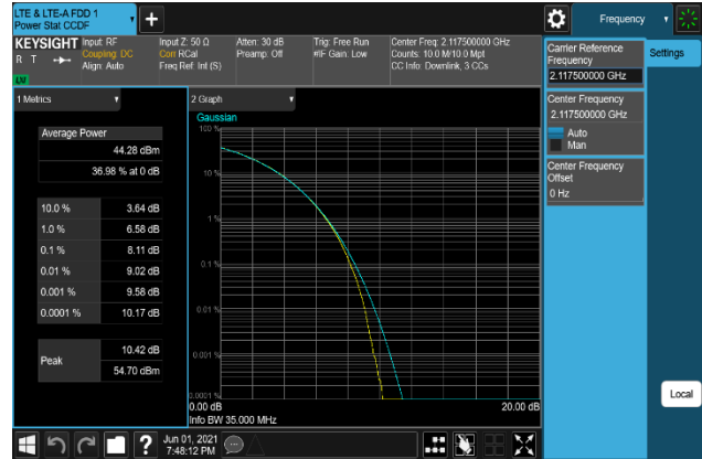
Plot 7-380. Peak To Average Power Ratio Plot (B66_15M+10M+10M_256QAM - Low Channel, Port 1)
