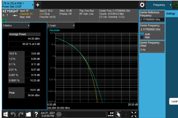
Plot 7-373. Peak To Average Power Ratio Plot (B66_15M+10M+10M_QPSK - Low Channel, Port 0)
