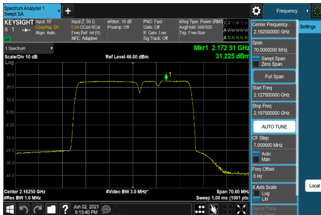
Plot 7-357. Peak To Average Power Ratio Plot (B66_20M+5M+10M_QPSK - High Channel, Port 0)
