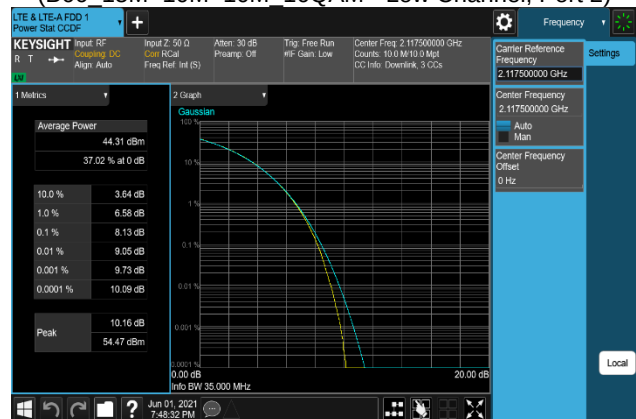
Plot 7-384. Peak To Average Power Ratio Plot (B66_15M+10M+10M_256QAM - Low Channel, Port 2)
