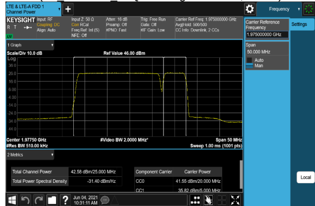
Plot 7-320. Conducted Average Output Power Plot (B2_20M+5M_256QAM - High Channel, Port 3)
