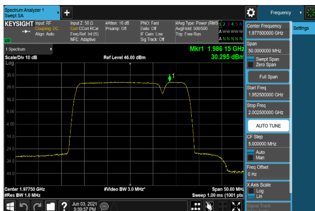
Plot 7-369. Peak To Average Power Ratio Plot (B2_20M+5M_QPSK - High Channel, Port 1)
