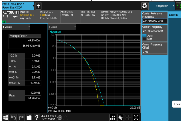
Plot 7-377. Peak To Average Power Ratio Plot (B66_15M+10M+10M_QPSK - Low Channel, Port 1)
