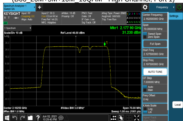
Plot 7-360. Peak To Average Power Ratio Plot (B66_20M+5M+10M_256QAM - High Channel, Port 0)
