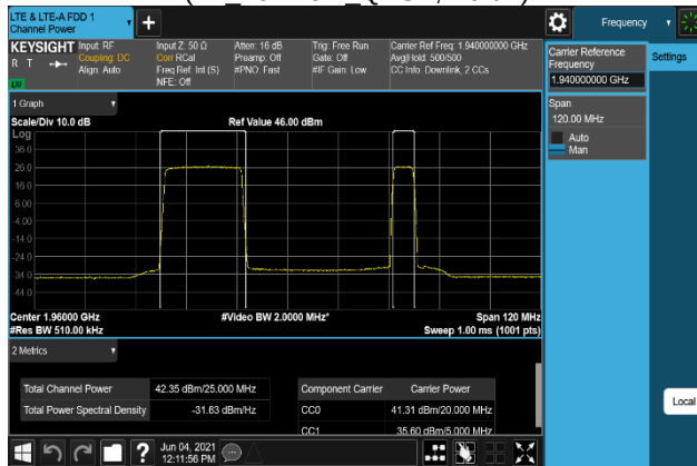
Plot 7-331. Conducted Average Output Power Plot (B2_20M+5M_64QAM, Port 2)
