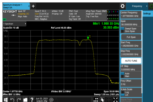
Plot 7-370. Peak To Average Power Ratio Plot (B2_20M+5M_16QAM - High Channel, Port 1)
