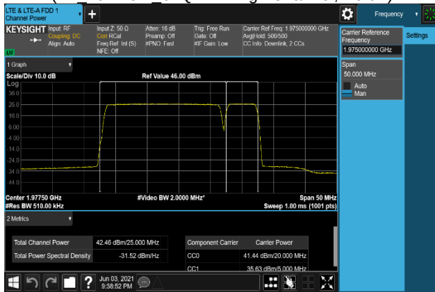
Plot 7-317. Conducted Average Output Power Plot (B2_20M+5M_QPSK - High Channel, Port 3)
