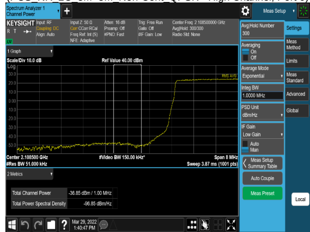
Plot 8-253. Band Edge Emission Plot (AWS_NR_1C_5M_64QAM - Low Channel, Port 1)
