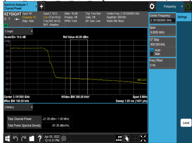
Plot 8-271. Band Edge Emission Plot (AWS DSS 5:5 1C 10M 256QAM - High Channel, Port 0)
