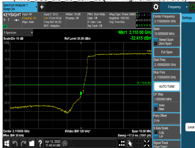
Plot 8-276. Band Edge Emission Plot (AWS_DSS_2:8_1C_20M_256QAM - Low Channel, Port 0)
