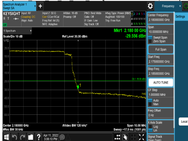
Plot 8-278. Band Edge Emission Plot (AWS_DSS_5:5_1C_20M_QPSK - High Channel, Port 0)
