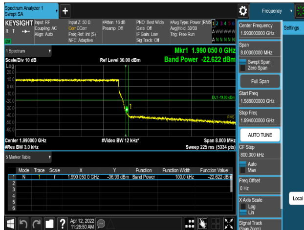
Plot 8-250. Band Edge Emission Plot (PCS_NR_2C_5M+5M_Non-Cont_QPSK - High Channel, Port 0)
