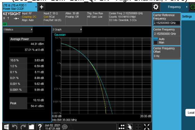
Plot 7-407. Peak To Average Power Radio Plot (B66_15M+10M+10M_64QAM - High Channel, Port 0)
