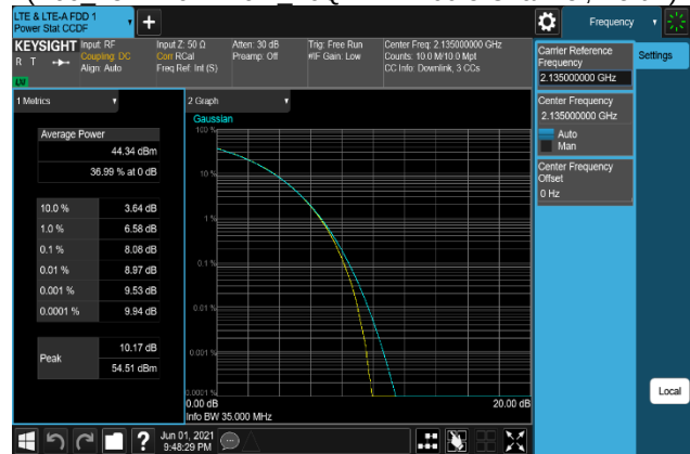
Plot 7-396. Peak To Average Power Ratio Plot (B66_15M+10M+10M_256QAM - Middle Channel, Port 1)
