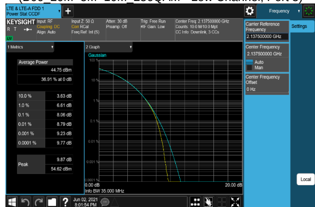
Plot 7-438. Peak To Average Power Ratio Plot (B66_20M+5M+10M_16QAM - Middle Channel, Port 0)
