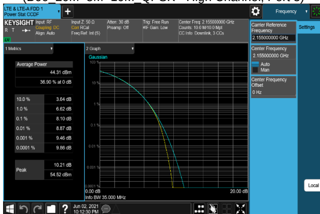
Plot 7-467. Peak To Average Power Ratio Plot (B66_20M+5M+10M_64QAM - High Channel, Port 3)
