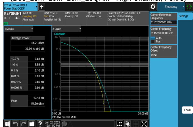
Plot 7-420. Peak To Average Power Radio Plot (B66_15M+10M+10M_256QAM - High Channel, Port 3)
