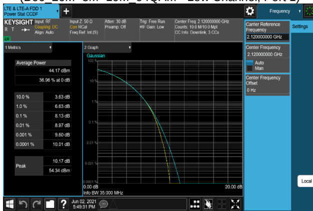
Plot 7-429. Peak To Average Power Ratio Plot (B66_20M+5M+10M_QPSK - Low Channel, Port 2)
