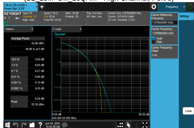
Plot 7-504. Peak To Average Power Ratio Plot (B2_20M+5M_256QAM - High Channel, Port 0)
