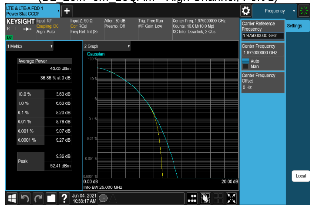
Plot 7-508. Peak To Average Power Ratio Plot (B2_20M+5M_256QAM - High Channel, Port 1)
