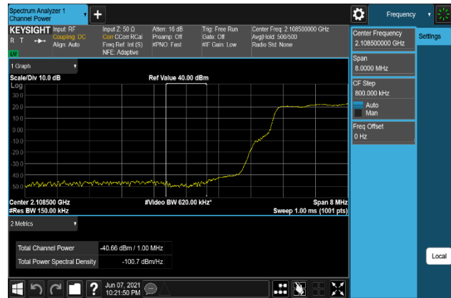
Plot 7-536. Band Edge Emission(Channel Power) Plot (B66_15M+10M+10M_16QAM - Low Channel, Port 2)
