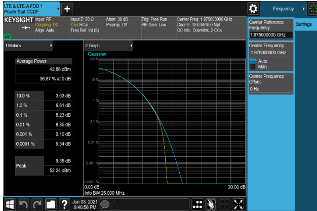
Plot 7-505. Peak To Average Power Ratio Plot (B2_20M+5M_QPSK - High Channel, Port 1)
