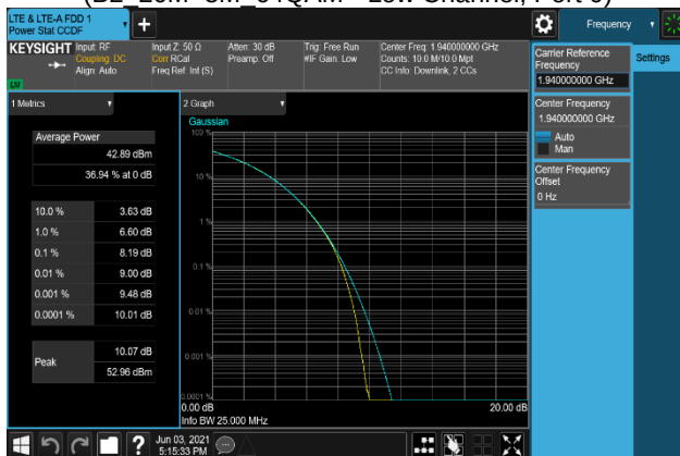
Plot 7-473. Peak To Average Power Ratio Plot (B2_20M+5M_QPSK - Low Channel, Port 1)
