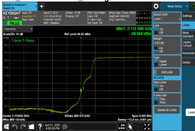
Plot 7-517. Band Edge Emission Plot (B66 15M+10M+10M QPSK - Low Channel, Port 0)
