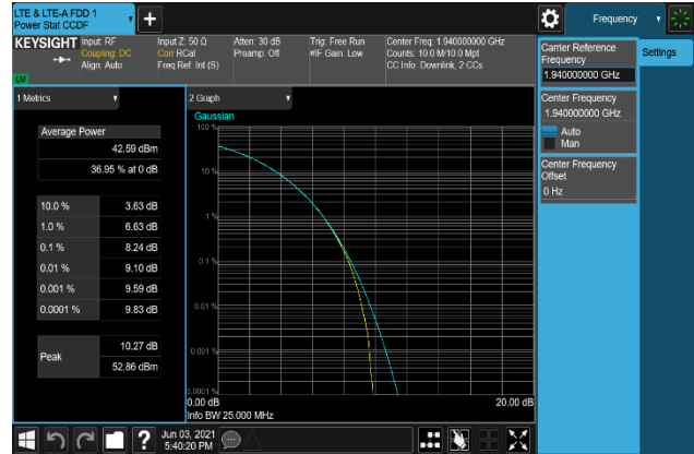
Plot 7-470. Peak To Average Power Ratio Plot (B2_20M+5M_16QAM - Low Channel, Port 0)
