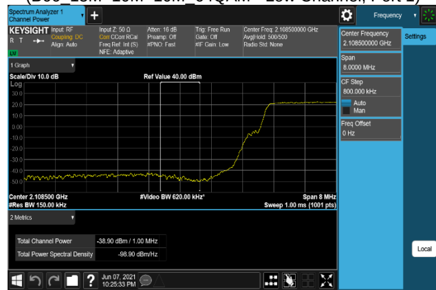
Plot 7-532. Band Edge Emission(Channel Power) Plot (B66_15M+10M+10M_256QAM - Low Channel, Port 1)
