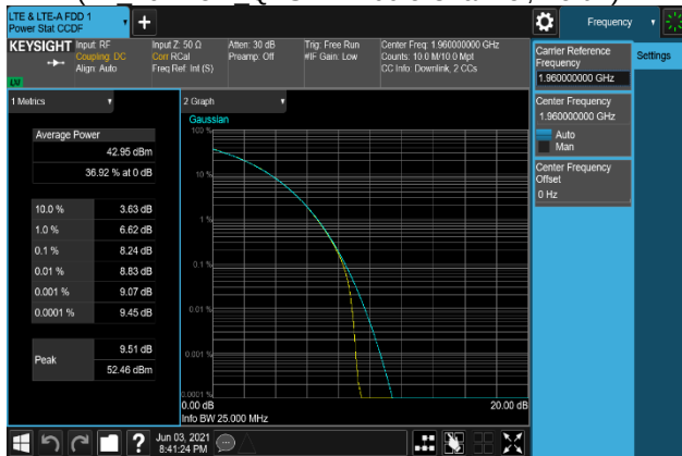
Plot 7-491. Peak To Average Power Ratio Plot (B2_20M+5M_64QAM - Middle Channel, Port 1)
