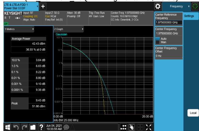
Plot 7-516. Peak To Average Power Radio Plot (B2_20M+5M_256QAM - High Channel, Port 3)
