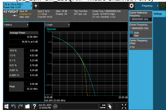
Plot 7-490. Peak To Average Power Ratio Plot (B2_20M+5M_16QAM - Middle Channel, Port 1)
