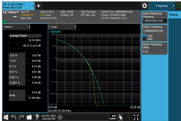
Plot 7-499. Peak To Average Power Ratio Plot (B2_20M+5M_64QAM - Middle Channel, Port 3)
