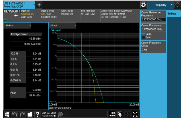
Plot 7-506. Peak To Average Power Ratio Plot (B2_20M+5M_16QAM - High Channel, Port 1)
