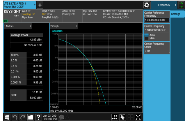
Plot 7-476. Peak To Average Power Ratio Plot (B2_20M+5M_256QAM - Low Channel, Port 1)
