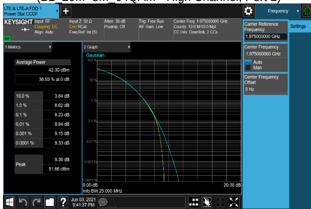
Plot 7-513. Peak To Average Power Radio Plot (B2_20M+5M_QPSK - High Channel, Port 3)
