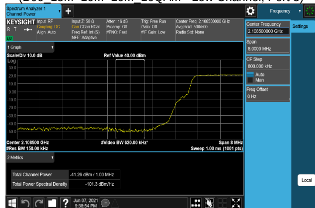
Plot 7-546. Band Edge Emission(Channel Power) Plot (B66_15M+10M+10M_64QAM - Low Channel, Port 3)
