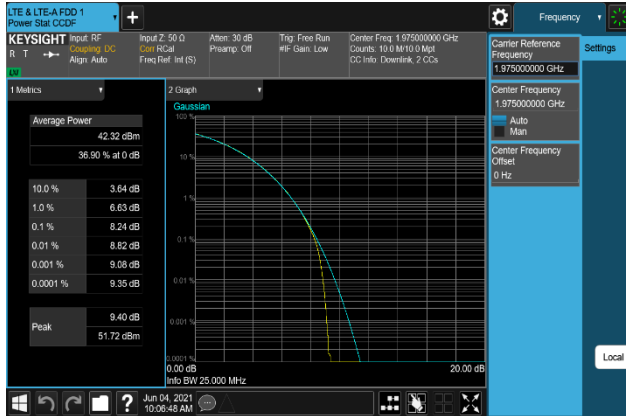
Plot 7-511. Peak To Average Power Radio Plot (B2_20M+5M_64QAM - High Channel, Port 2)
