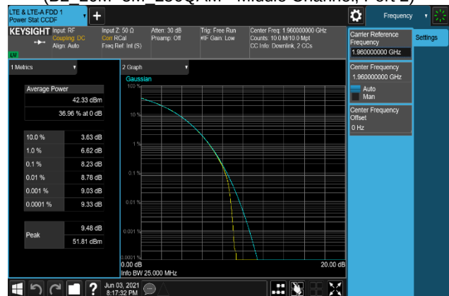
Plot 7-498. Peak To Average Power Ratio Plot (B2_20M+5M_16QAM - Middle Channel, Port 3)
