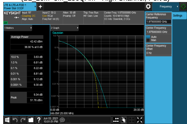
Plot 7-514. Peak To Average Power Radio Plot (B2_20M+5M_16QAM - High Channel, Port 3)
