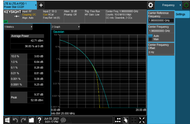
Plot 7-488. Peak To Average Power Ratio Plot (B2_20M+5M_256QAM - Middle Channel, Port 0)
