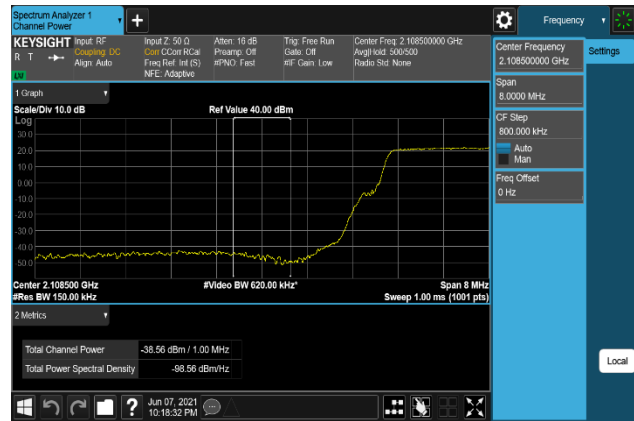
Plot 7-518. Band Edge Emission(Channel Power) Plot (B66 15M+10M+10M QPSK - Low Channel, Port 0)
