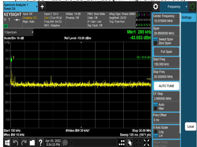
Plot 8-345. Conducted Spurious Emission Plot 150 kHz to 30 MHz (AWS_NR_2C_15M + 20M_QPSK - Mid Channel, Port 0)
