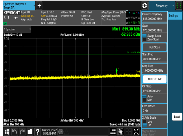
Plot 8-325. Conducted Spurious Emission Plot 30 MHz to 1 GHz (AWS NR 1C 5M 16QAM - High Channel, Port 2)
