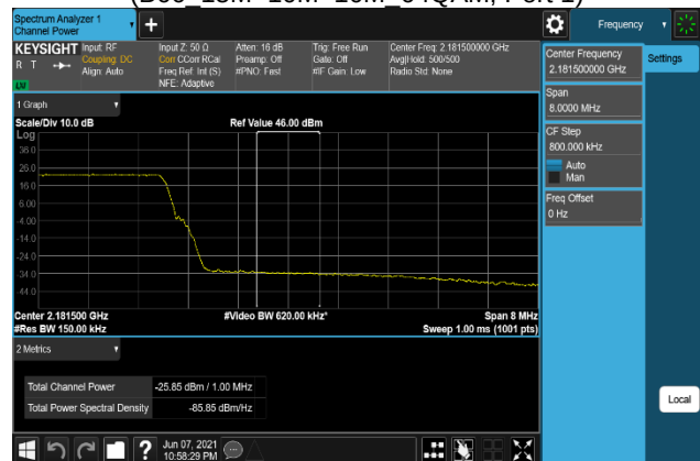
Plot 7-628. Band Edge Emission(Channel Power) Plot (B66_15M+10M+10M_256QAM, Port 1)
