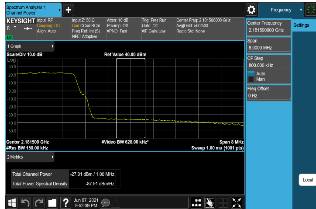
Plot 7-560. Band Edge Emission(Channel Power) Plot (B66_15M+10M+10M_16QAM - High Channel, Port 1)
