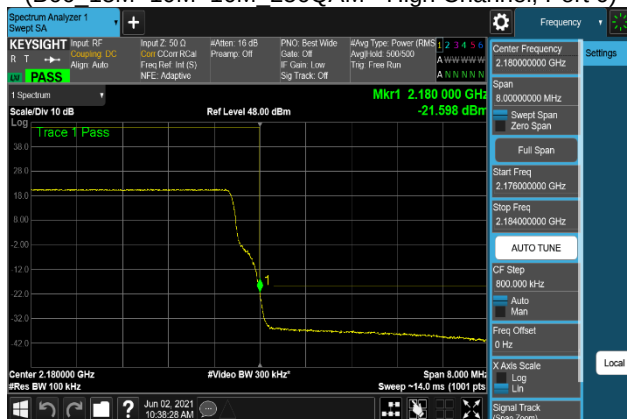
Plot 7-557. Band Edge Emission Plot (B66_15M+10M+10M_QPSK - High Channel, Port 1)
