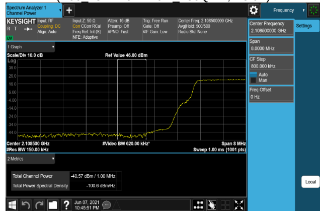
Plot 7-598. Band Edge Emission(Channel Power) Plot (B66_15M+10M+10M_QPSK, Port 2)
