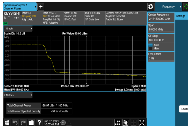
Plot 7-578. Band Edge Emission(Channel Power) Plot (B66_15M+10M+10M_64QAM - High Channel, Port 3)
