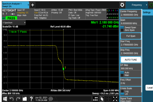
Plot 7-553. Band Edge Emission Plot (B66_15M+10M+10M_64QAM - High Channel, Port 0)
