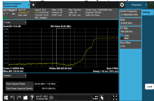
Plot 7-596. Band Edge Emission(Channel Power) Plot (B66_15M+10M+10M_256QAM, Port 1)
