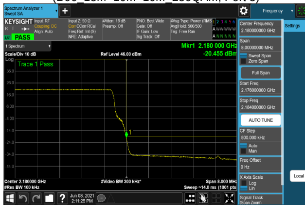
Plot 7-613. Band Edge Emission Plot (B66_15M+10M+10M_QPSK, Port 0)
