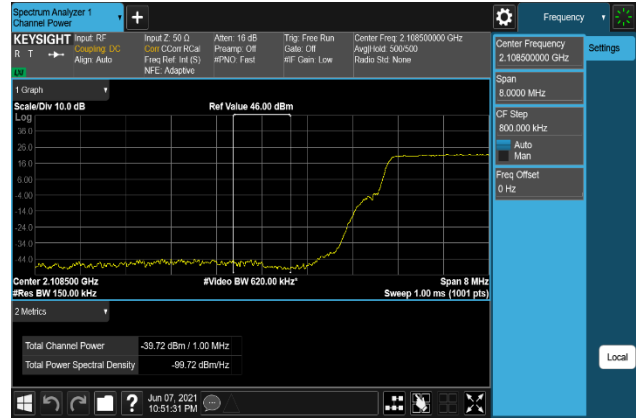
Plot 7-594. Band Edge Emission(Channel Power) Plot (B66_15M+10M+10M_64QAM, Port 1)
