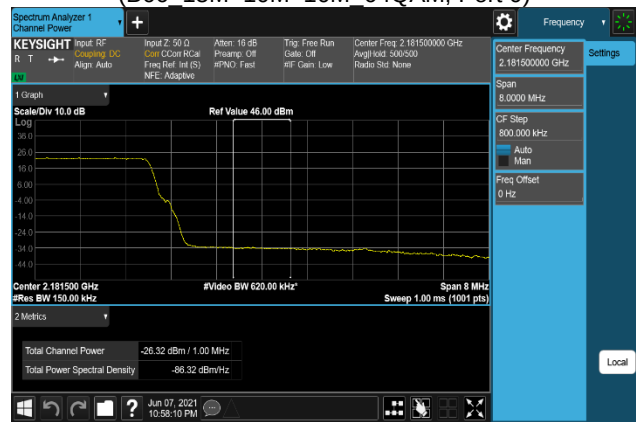
Plot 7-620. Band Edge Emission(Channel Power) Plot (B66_15M+10M+10M_256QAM, Port 0)
