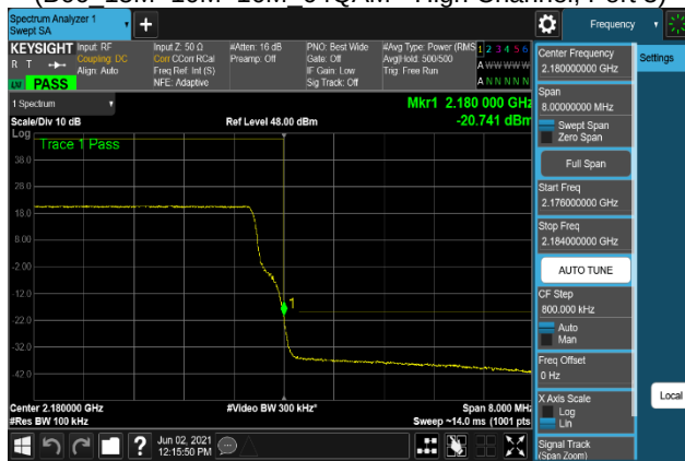
Plot 7-579. Band Edge Emission Plot (B66_15M+10M+10M_256QAM - High Channel, Port 3)
