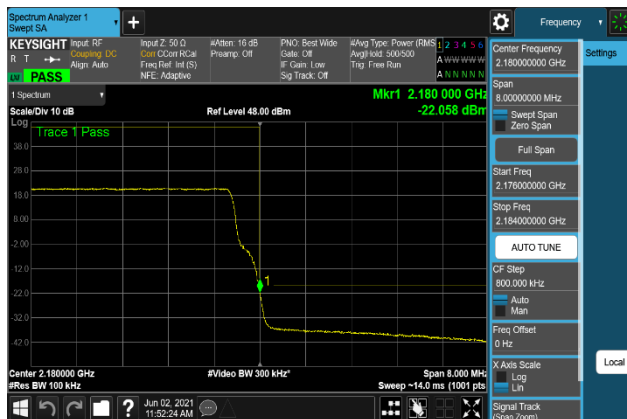
Plot 7-577. Band Edge Emission Plot (B66_15M+10M+10M_64QAM - High Channel, Port 3)
