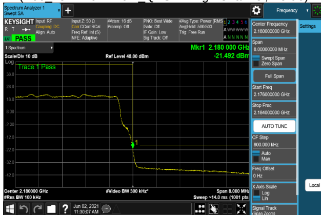
Plot 7-551. Band Edge Emission Plot (B66_15M+10M+10M_16QAM - High Channel, Port 0)
