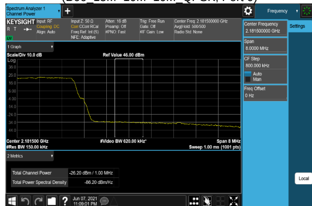
Plot 7-616. Band Edge Emission(Channel Power) Plot (B66_15M+10M+10M_16QAM, Port 0)
