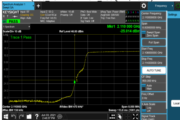
Plot 7-597. Band Edge Emission Plot (B66_15M+10M+10M_QPSK, Port 2)
