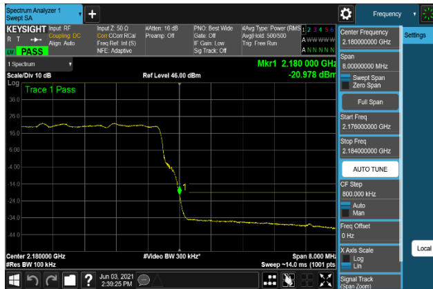
Plot 7-623. Band Edge Emission Plot (B66 15M+10M+10M 16QAM, Port 1)
