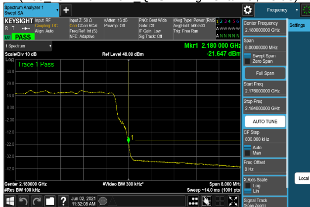
Plot 7-575. Band Edge Emission Plot (B66_15M+10M+10M_16QAM - High Channel, Port 3)
