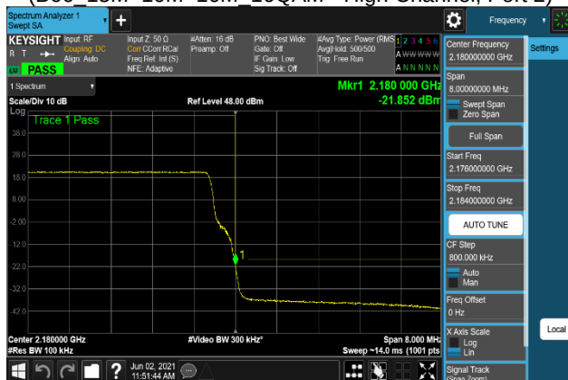
Plot 7-569. Band Edge Emission Plot (B66_15M+10M+10M_64QAM - High Channel, Port 2)
