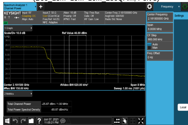
Plot 7-614. Band Edge Emission(Channel Power) Plot (B66_15M+10M+10M_QPSK, Port 0)
