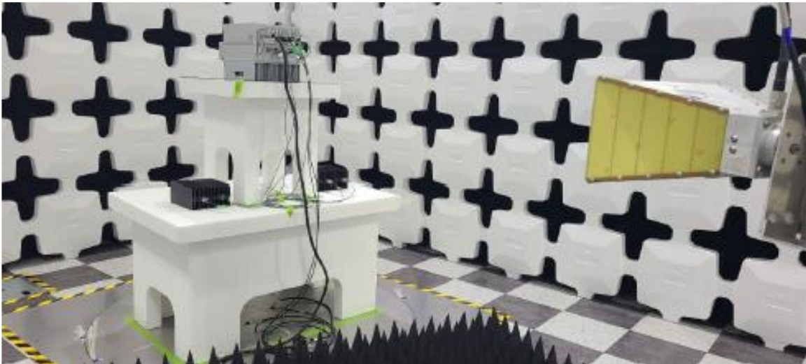
Above 1GHz Radiated spurious emission Measurement Setup > 1GHz
