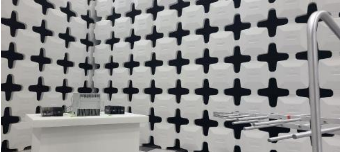
Below 1GHz Radiated spurious emission Measurement Setup
