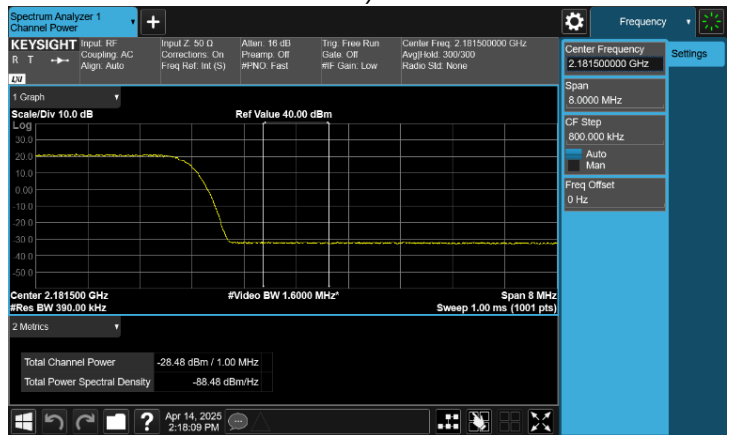
Plot 8-127. Conducted Spurious Emission Plot 2.181 GHz to 2.182 GHz (B/n66(B/n4)_NC_NR_1C_25M+LTE_2C_10M+5M - QPSK, Port 2)
