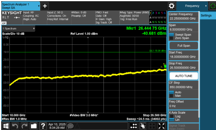
Plot 8-103. Conducted Spurious Emission Plot 18 GHz to 26.5 GHz (n66(n4)_NR_1C_30M_256QAM - High Channel, Port 3)
