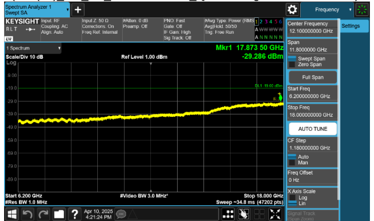
Plot 8-111. Conducted Spurious Emission Plot 6.2 GHz to 18 GHz
