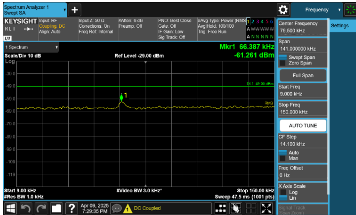
Plot 8-86. Conducted Spurious Emission Plot 9 kHz to 150 kHz
