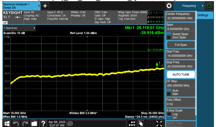
Plot 8-85. Conducted Spurious Emission Plot 18 GHz to 26.5 GHz (n25(n2)_NR_2NC_5M+25M_QPSK, Port 1)
