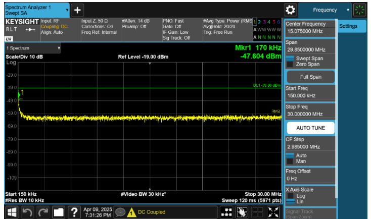
Plot 8-87. Conducted Spurious Emission Plot 150 kHz to 30 MHz
