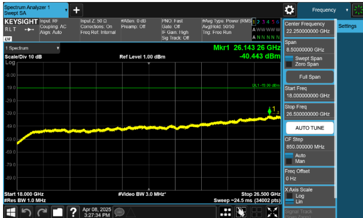
Plot 8-75. Conducted Spurious Emission Plot 18 GHz to 26.5 GHz (n25(n2)_NR_1C_25M + LTE_1C_5M_QPSK - High Channel, Port 2)
