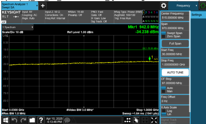
Plot 8-106. Conducted Spurious Emission Plot 30 MHz to 1 GHz (n66(n4)_NR_3C_5M+10M+25M_QPSK - High Channel, Port 0)
