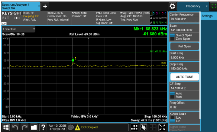
Plot 8-104. Conducted Spurious Emission Plot 9 kHz to 150 kHz (n66(n4)_NR_3C_5M+10M+25M_QPSK - High Channel, Port 0)
