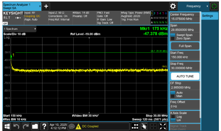
Plot 8-105. Conducted Spurious Emission Plot 150 kHz to 30 MHz (n66(n4)_NR_3C_5M+10M+25M_QPSK - High Channel, Port 0)
