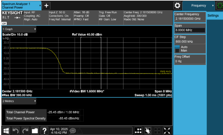
Plot 8-108. Conducted Spurious Emission Plot 2.181 GHz to 2.182 GHz
