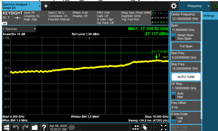
Plot 8-84. Conducted Spurious Emission Plot 6.2 GHz to 18 GHz (n25(n2)_NR_2NC_5M+25M_QPSK, Port 1)
