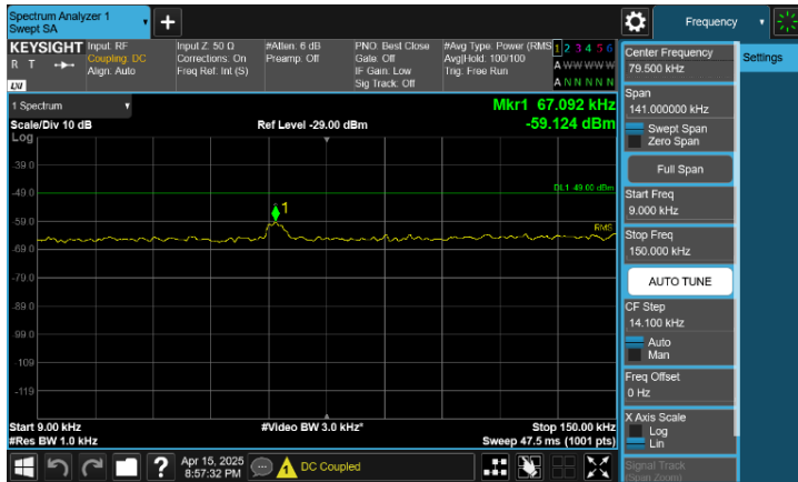
Plot 8-113. Conducted Spurious Emission Plot 9 kHz to 150 kHz (B/n66(B/n4)_NR_1C_25M+DSS_1C_15M_QPSK - High Channel, Port 1)
