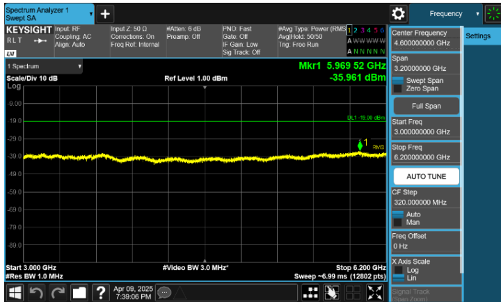
Plot 8-92. Conducted Spurious Emission Plot 3 GHz to 6.2 GHz
