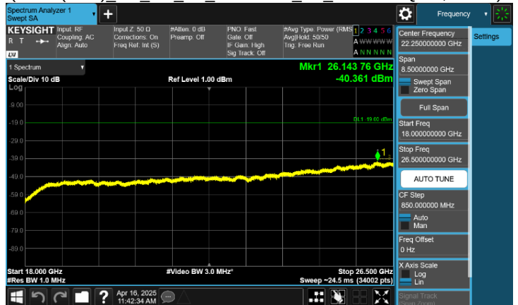
Plot 8-141. Conducted Spurious Emission Plot 18 GHz to 26.5 GHz
