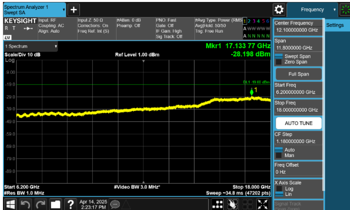
Plot 8-130. Conducted Spurious Emission Plot 6.2 GHz to 18 GHz (B/n66(B/n4)_NC_NR_1C_25M+LTE_2C_10M+5M - QPSK, Port 2)
