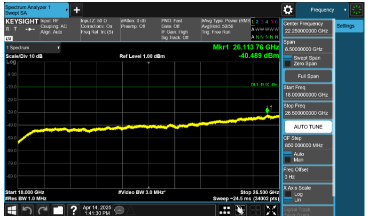
Plot 8-131. Conducted Spurious Emission Plot 18 GHz to 26.5 GHz (B/n66(B/n4)_NC_NR_1C_25M+LTE_2C_10M+5M - QPSK, Port 2)
