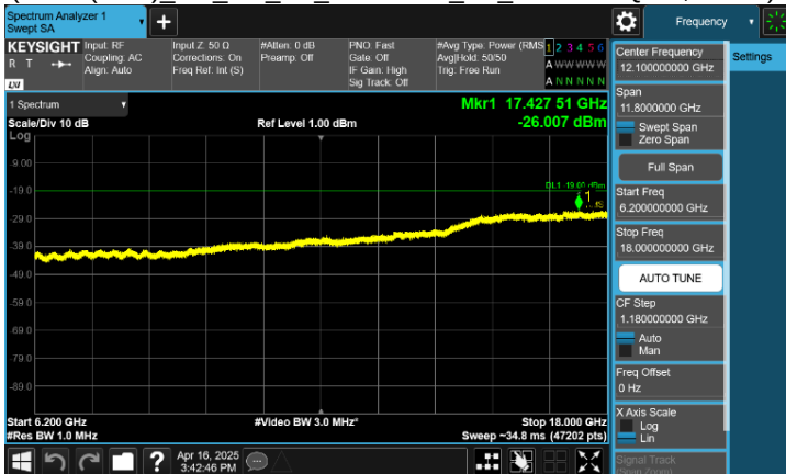
Plot 8-140. Conducted Spurious Emission Plot 6.2 GHz to 18 GHz
