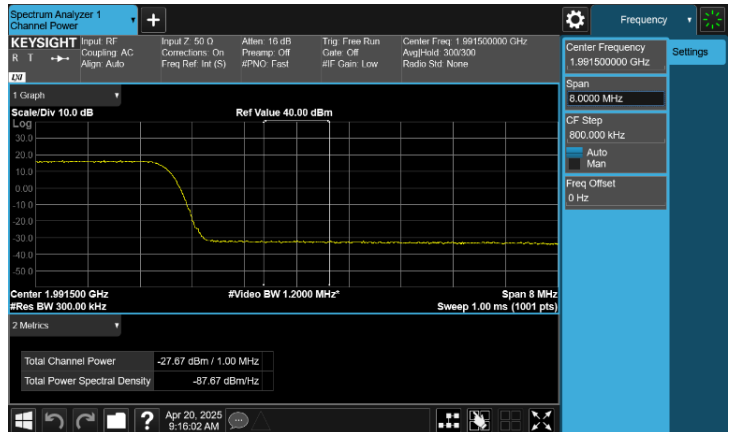
Plot 8-160. Conducted Spurious Emission Plot 1.991 MHz to 1.992 GHz
