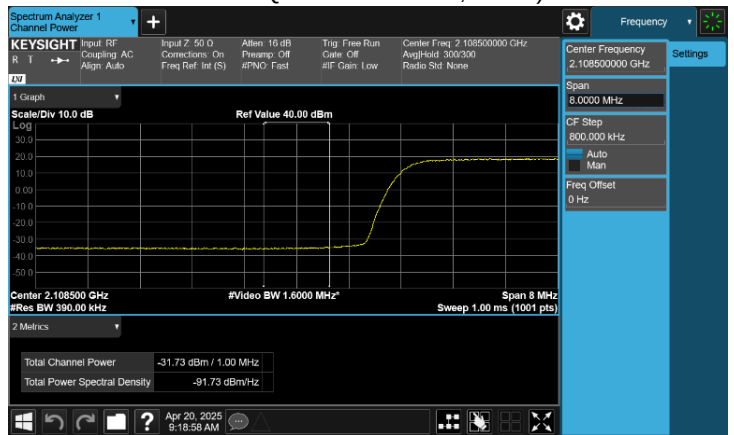
Plot 8-162. Conducted Spurious Emission Plot 2.108 MHz to 2.109 GHz
