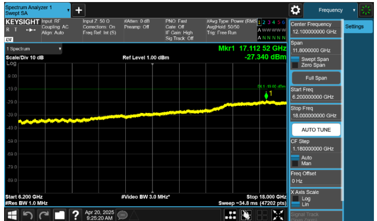
Plot 8-166. Conducted Spurious Emission Plot 6.2 GHz to 18 GHz
