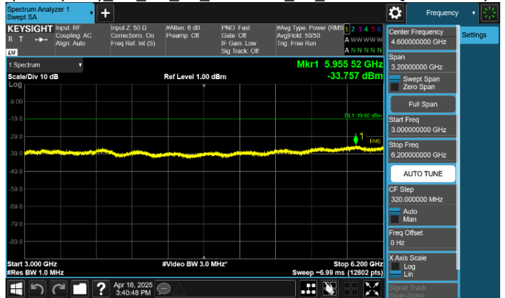
Plot 8-139. Conducted Spurious Emission Plot 3 GHz to 6.2 GHz
