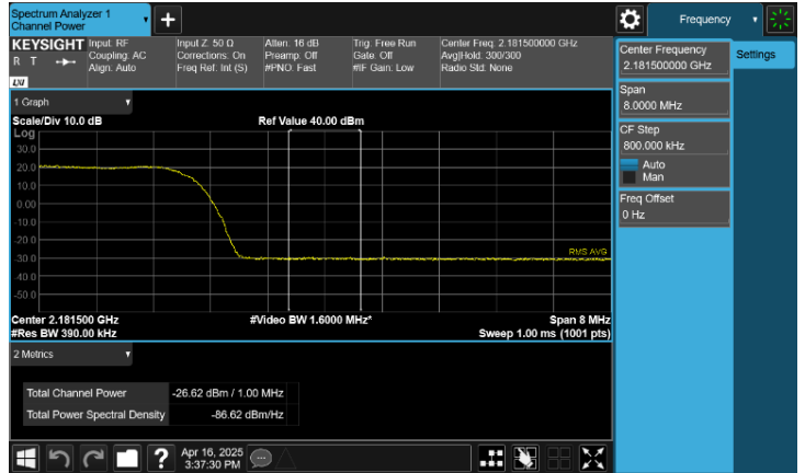
Plot 8-137. Conducted Spurious Emission Plot 2.181 GHz to 2.182 GHz
