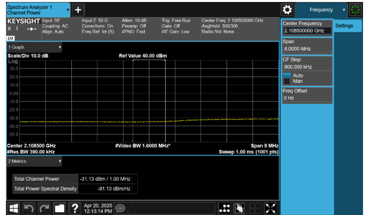
Plot 8-149. Conducted Spurious Emission Plot 2.108 GHz to 2.109 GHz (n25(n2)_NR_3C_5M+5M+20M+B/n66(B/n4)_NR_2C_10M+30M_16QAM – Multi-Band, Port 1)
