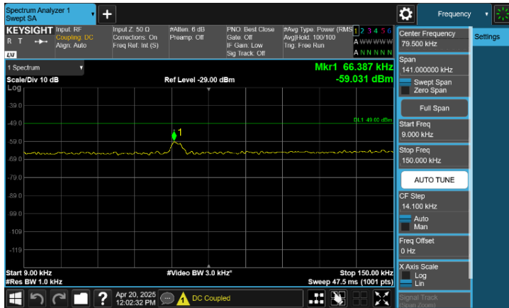
Plot 8-142. Conducted Spurious Emission Plot 9 kHz to 150 kHz
