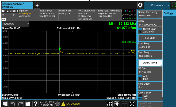
Plot 8-132. Conducted Spurious Emission Plot 9 kHz to 150 kHz (B/n66(B/n4)_NC_NR_1C_25M+DSS_1C_15M - 16QAM, Port 3)
