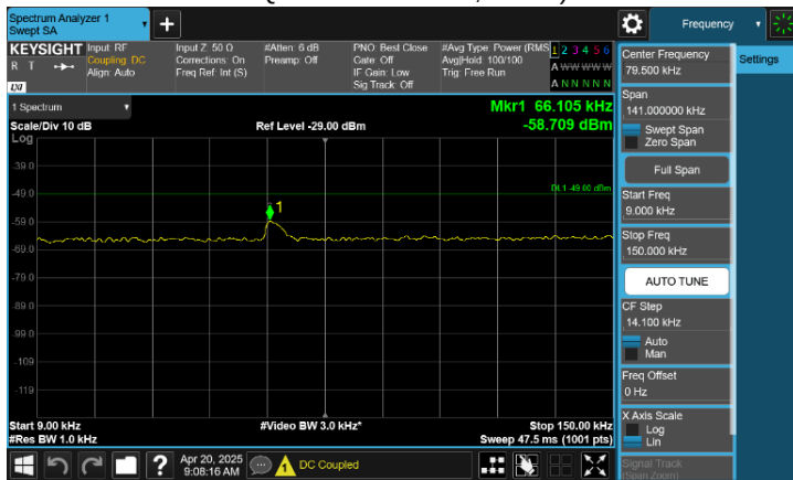
Plot 8-155. Conducted Spurious Emission Plot 9 kHz to 150 kHz
