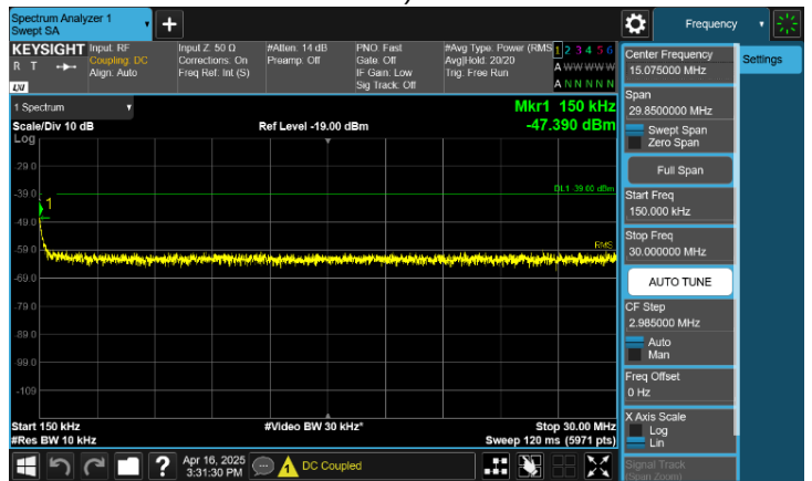
Plot 8-133. Conducted Spurious Emission Plot 150 kHz to 30 MHz (B/n66(B/n4)_NC_NR_1C_25M+DSS_1C_15M - 16QAM, Port 3)
