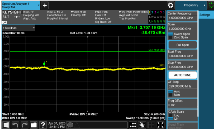
Plot 8-64. Conducted Spurious Emission Plot 3 GHz to 6.2 GHz
