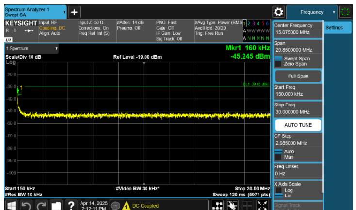
Plot 8-123. Conducted Spurious Emission Plot 150 kHz to 30 MHz (B/n66(B/n4)_NC_NR_1C_25M+LTE_2C_10M+5M - QPSK, Port 2)
