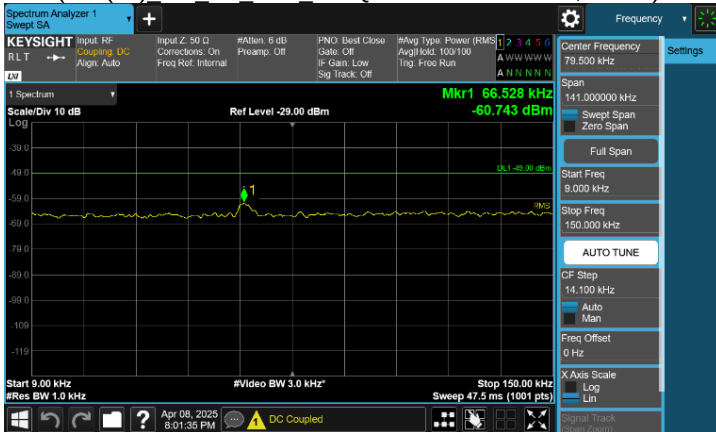
Plot 8-67. Conducted Spurious Emission Plot 9 kHz to 150 kHz
