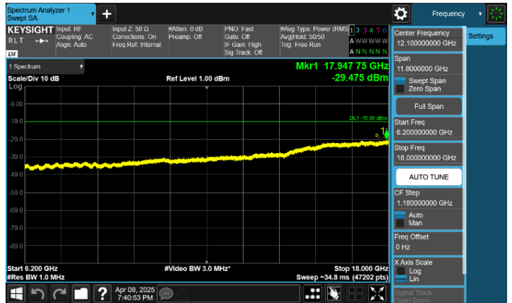
Plot 8-93. Conducted Spurious Emission Plot 6.2 GHz to 18 GHz
