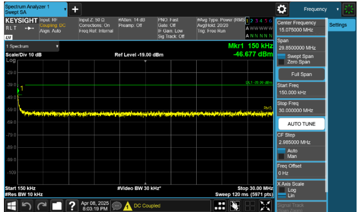
Plot 8-68. Conducted Spurious Emission Plot 150 kHz to 30 MHz
