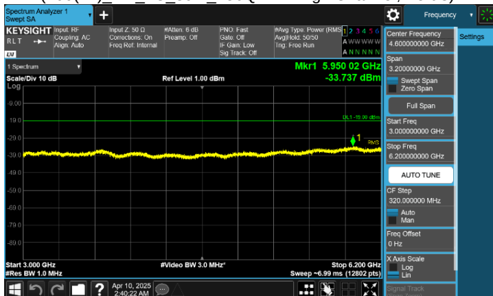
Plot 8-101. Conducted Spurious Emission Plot 3 GHz to 6.2 GHz
