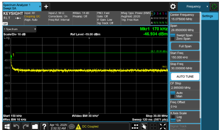
Plot 8-96. Conducted Spurious Emission Plot 150 kHz to 30 MHz
