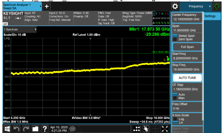
Plot 8-111. Conducted Spurious Emission Plot 6.2 GHz to 18 GHz
