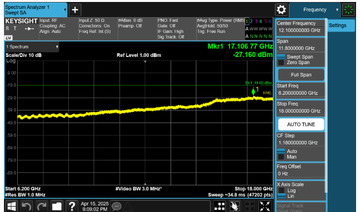
Plot 8-120. Conducted Spurious Emission Plot 6.2 GHz to 18 GHz (B/n66(B/n4)_NR_1C_25M+DSS_1C_15M_QPSK - High Channel, Port 1)
