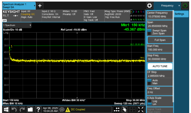
Plot 8-77. Conducted Spurious Emission Plot 150 kHz to 30 MHz (n25(n2)_NR_2NC_5M+25M_QPSK, Port 1)
