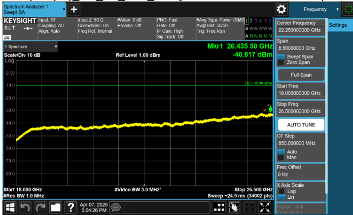
Plot 8-66. Conducted Spurious Emission Plot 18 GHz to 26.5 GHz
