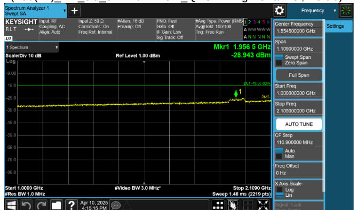
Plot 8-107. Conducted Spurious Emission Plot 1 GHz to 2.109 GHz (n66(n4)_NR_3C_5M+10M+25M_QPSK - High Channel, Port 0)
