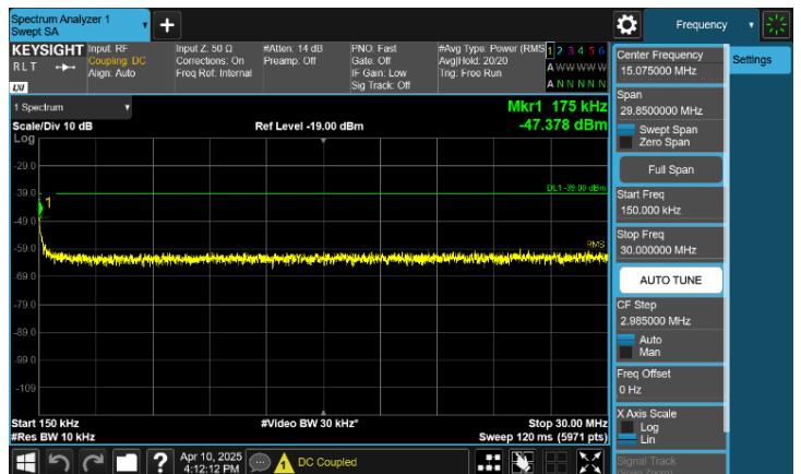
Plot 8-105. Conducted Spurious Emission Plot 150 kHz to 30 MHz (n66(n4)_NR_3C_5M+10M+25M_QPSK - High Channel, Port 0)
