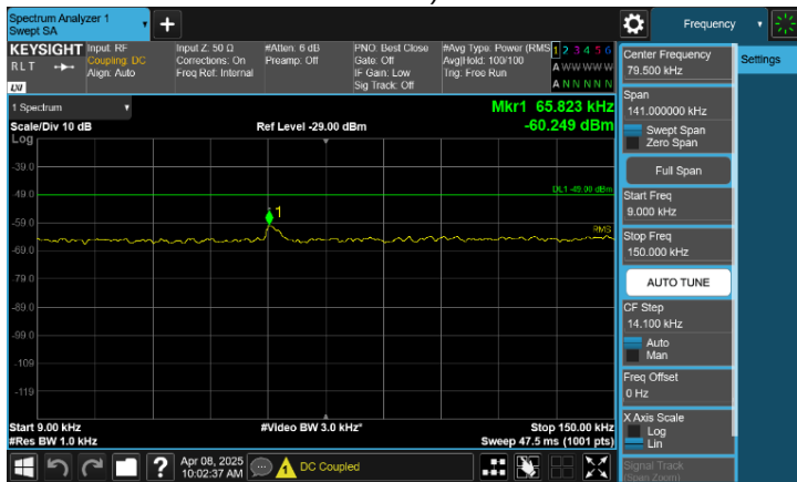
Plot 8-76. Conducted Spurious Emission Plot 9 kHz to 150 kHz (n25(n2)_NR_2NC_5M+25M_QPSK, Port 1)
