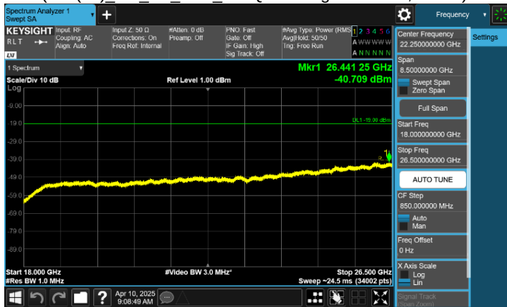
Plot 8-94. Conducted Spurious Emission Plot 18 GHz to 26.5 GHz
