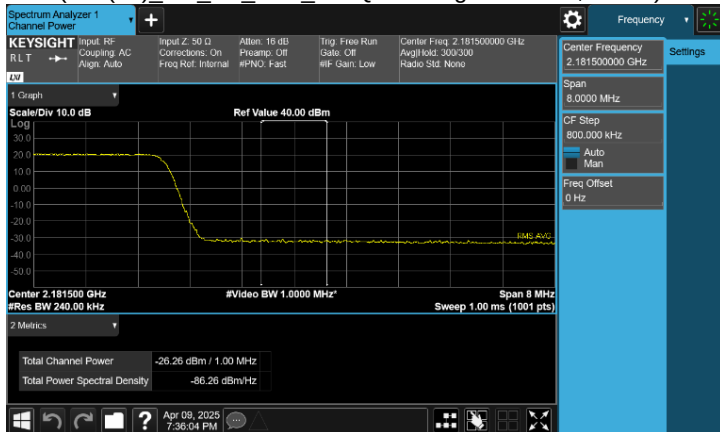
Plot 8-90. Conducted Spurious Emission Plot 2.181 GHz to 2.182 GHz
