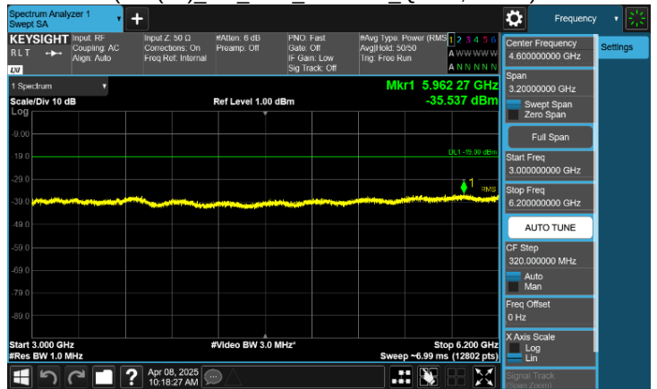
Plot 8-83. Conducted Spurious Emission Plot 3 GHz to 6.2 GHz (n25(n2)_NR_2NC_5M+25M_QPSK, Port 1)
