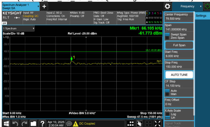
Plot 8-95. Conducted Spurious Emission Plot 9 kHz to 150 kHz
