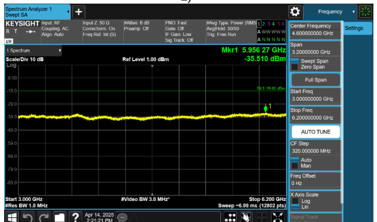
Plot 8-129. Conducted Spurious Emission Plot 3 GHz to 6.2 GHz (B/n66(B/n4)_NC_NR_1C_25M+LTE_2C_10M+5M - QPSK, Port 2)
