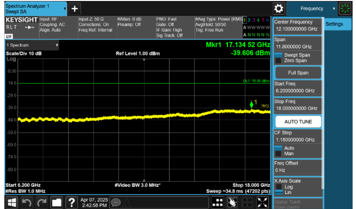
Plot 8-65. Conducted Spurious Emission Plot 6.2 GHz to 18 GHz
