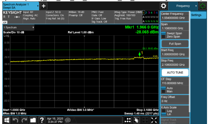
Plot 8-135. Conducted Spurious Emission Plot 1 GHz to 2.108 GHz (B/n66(B/n4)_NC_NR_1C_25M+DSS_1C_15M - 16QAM, Port 3)
