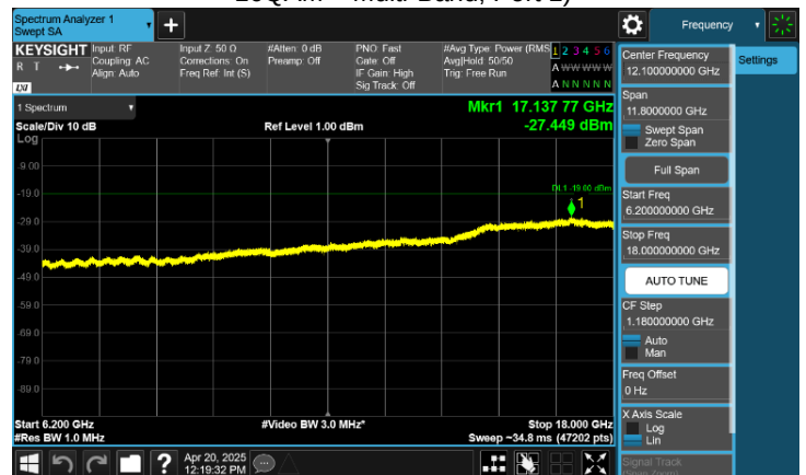
Plot 8-153. Conducted Spurious Emission Plot 6.2 GHz to 18 GHz (n25(n2)_NR_3C_5M+5M+20M+B/n66(B/n4)_NR_2C_10M+30M_16QAM – Multi-Band, Port 1)
