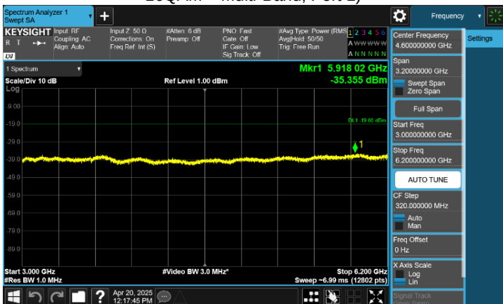
Plot 8-152. Conducted Spurious Emission Plot 3 GHz to 6.2 GHz (n25(n2)_NR_3C_5M+5M+20M+B/n66(B/n4)_NR_2C_10M+30M_16QAM – Multi-Band, Port 1)
