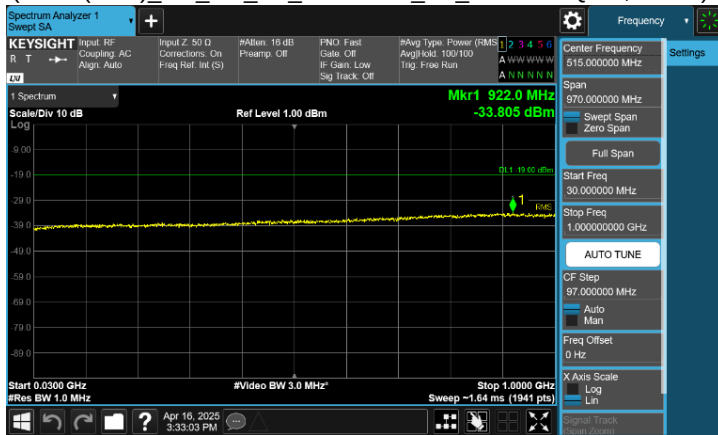
Plot 8-134. Conducted Spurious Emission Plot 30 MHz to 1 GHz (B/n66(B/n4)_NC_NR_1C_25M+DSS_1C_15M - 16QAM, Port 3)
