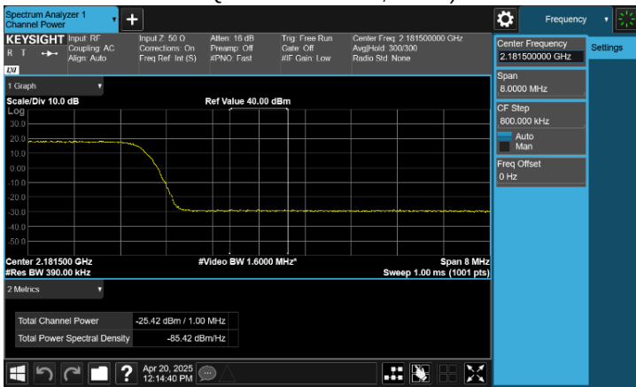
Plot 8-150. Conducted Spurious Emission Plot 2.181 GHz to 2.182 GHz (n25(n2)_NR_3C_5M+5M+20M+B/n66(B/n4)_NR_2C_10M+30M_16QAM – Multi-Band, Port 1)
