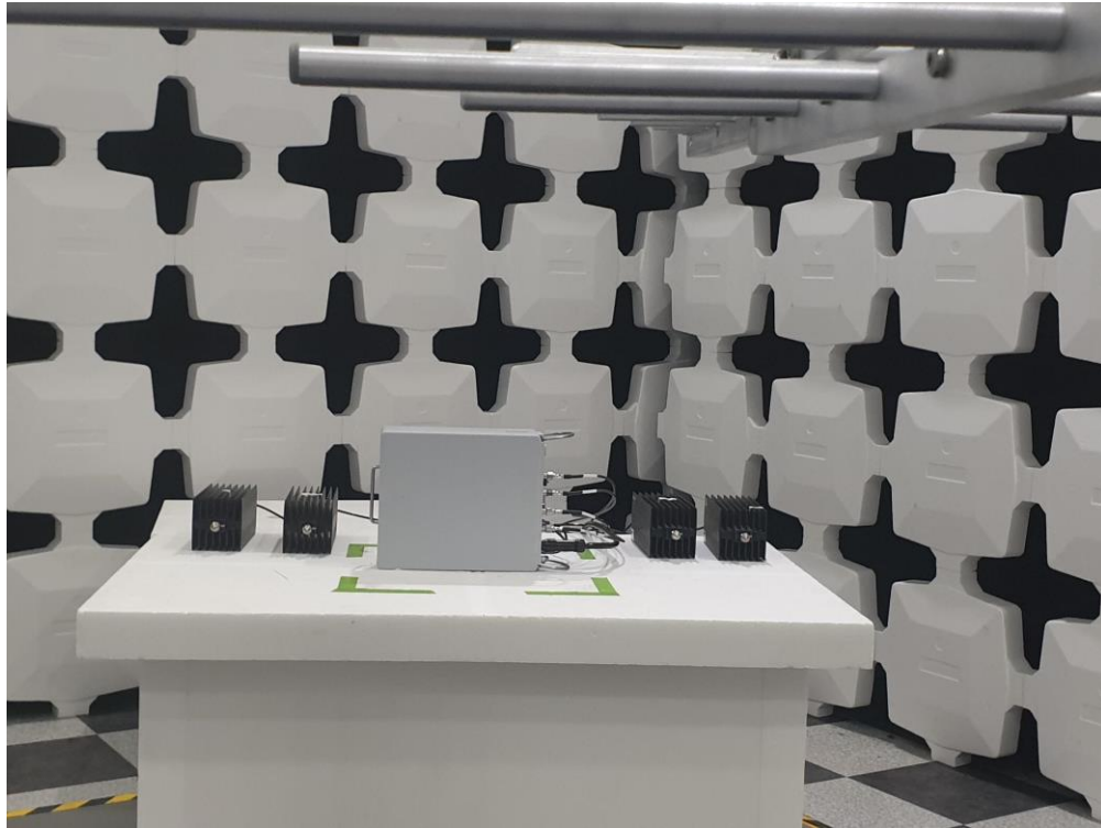
Testing setup for 30 MHz to 1 GHz
