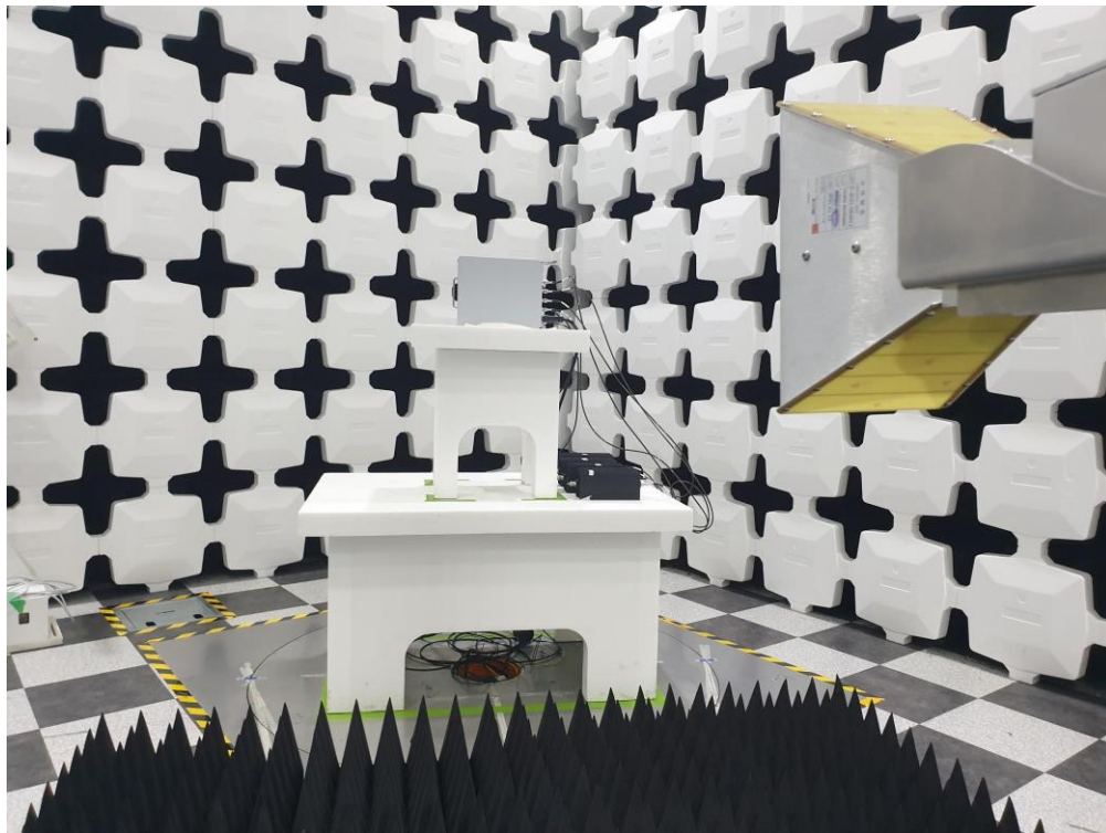
Testing setup for 1 GHz to 18 GHz
