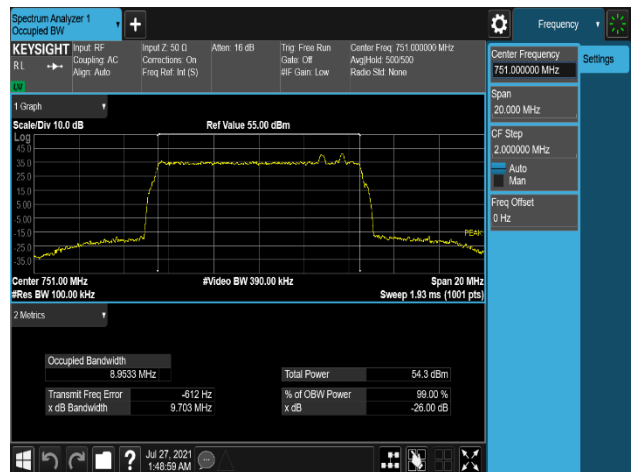
Plot 7-156. Occupied Bandwidth Plot (B13_10M+High_NB-lot(IB)+High_NB-lot(IB)_1C_QPSK - Port 3)
