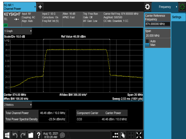
Plot 7-400. Conducted Average Output Power Plot (B5_10M(DSS_8:2) 1C_QPSK - Low Channel, Port 3)
