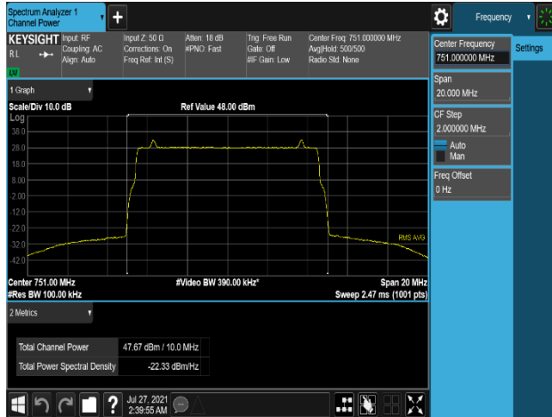
Plot 7-361. Conducted Average Output Power Plot (B13_10M+Low_NB-lot(IB)+High_NB-lot(IB)_1C - Port 0)
