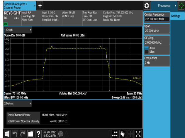
Plot 7-368. Conducted Average Output Power Plot (B13_10M+Low_NB-lot(IB)+High_NB-lot(IB)_1C - Port 1)
