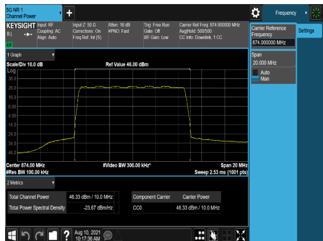
Plot 7-402. Conducted Average Output Power Plot (B5_10M(DSS_7:3) 1C_16QAM - Low Channel, Port 1)
