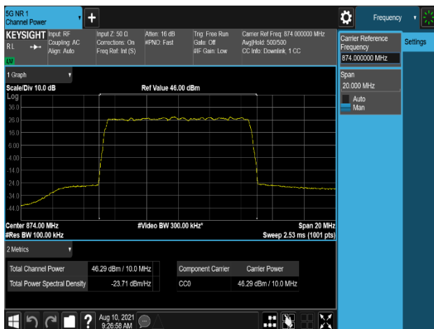
Plot 7-407. Conducted Average Output Power Plot (B5_10M(DSS_8:2) 1C_64QAM - Low Channel, Port 2)
