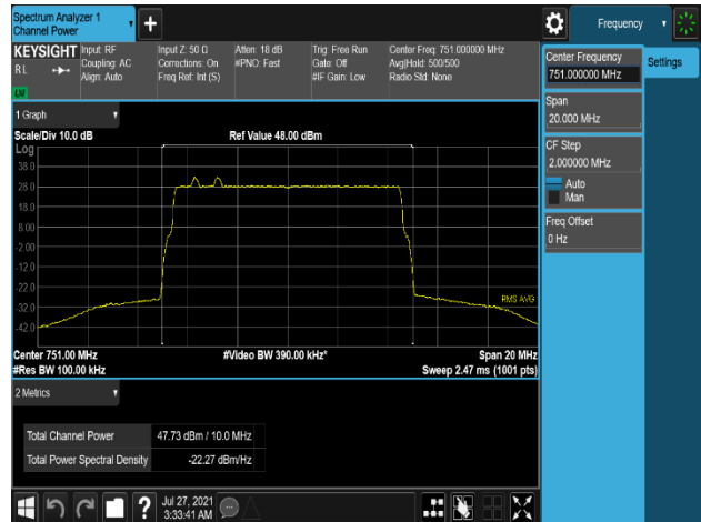
Plot 7-364. Conducted Average Output Power Plot (B13_10M+Low_NB-lot(IB)+Low_NB-lot(IB)_1C - Port 1)
