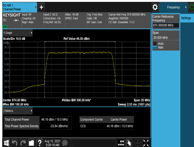
Plot 7-405. Conducted Average Output Power Plot (B5_10M(DSS_8:2) 1C_64QAM - Low Channel, Port 0)
