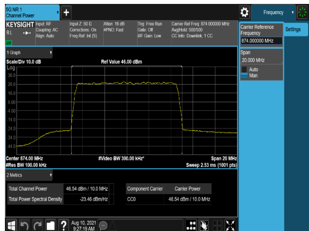
Plot 7-408. Conducted Average Output Power Plot (B5_10M(DSS_8:2) 1C_64QAM - Low Channel, Port 3)
