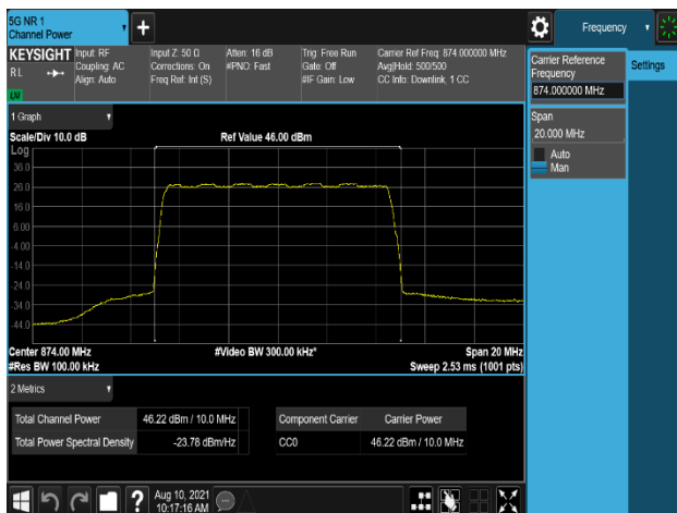
Plot 7-401. Conducted Average Output Power Plot (B5_10M(DSS_7:3) 1C_16QAM - Low Channel, Port 0)
