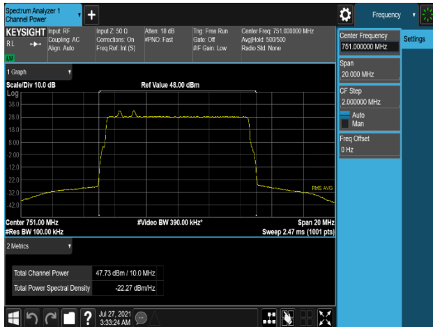
Plot 7-363. Conducted Average Output Power Plot (B13_10M+Low_NB-lot(IB)+Low_NB-lot(IB)_1C - Port 0)
