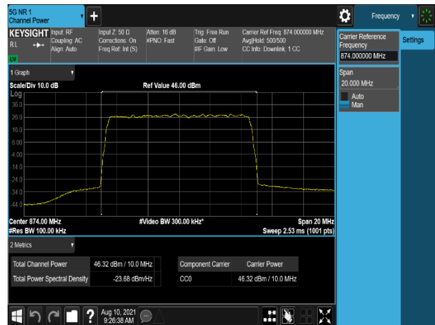
Plot 7-406. Conducted Average Output Power Plot (B5_10M(DSS_8:2) 1C_64QAM - Low Channel, Port 1)
