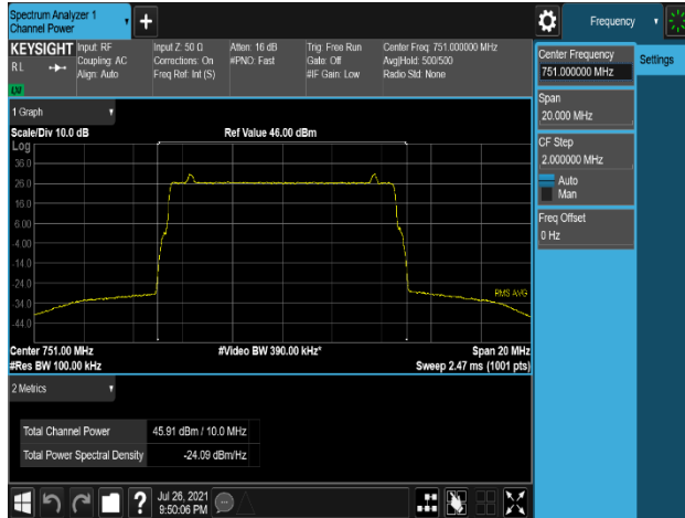
Plot 7-367. Conducted Average Output Power Plot (B13_10M+Low_NB-lot(IB)+High_NB-lot(IB)_1C - Port 0)
