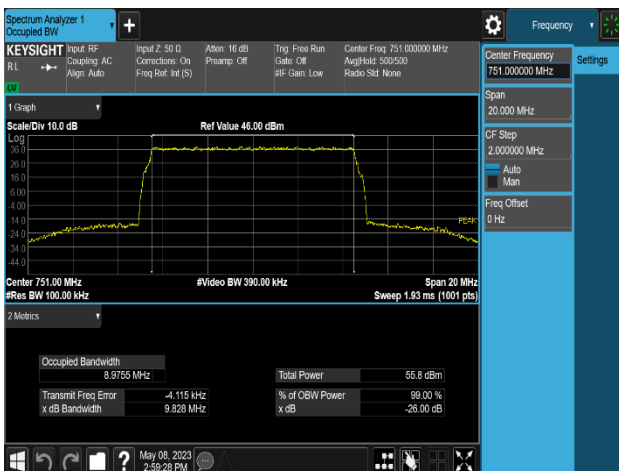
Plot 8-41. Occupied Bandwidth Plot (LTE B13_1C_10M_QPSK - Mid Channel_2T, Port 1)
