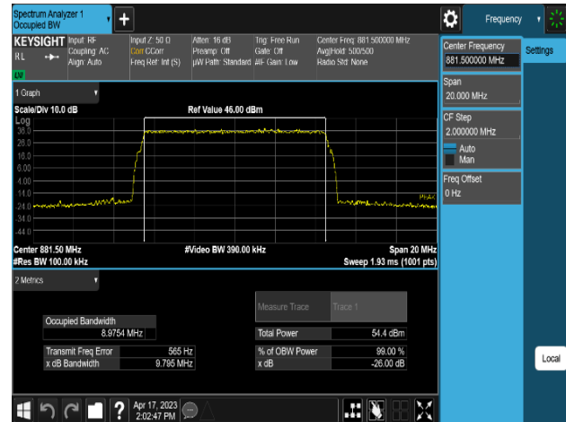
Plot 8-50. Occupied Bandwidth Plot (LTE B5_1C_10M_64QAM - Mid Channel_4T, Port 1)
