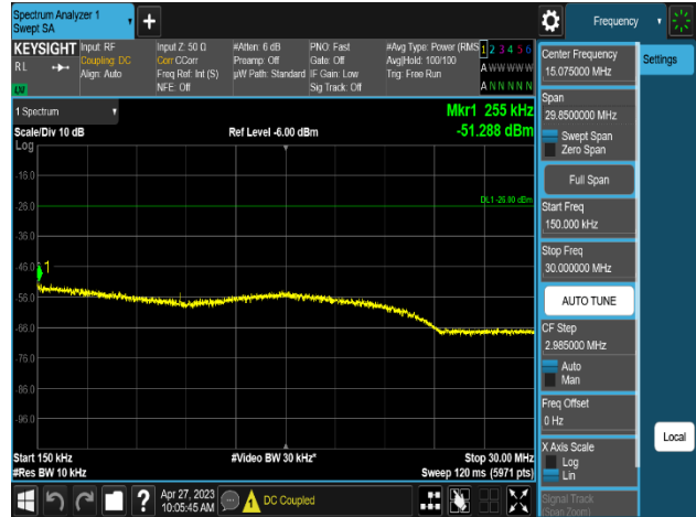
Plot 8-568. Conducted Spurious Emission Plot 150 kHz to 30 MHz (MSR 3NC_DSS B(n)5_1C_10M+NR n5_1C_5M+LTE B5_1C_5M_2T_QPSK-Mid Channel, Port 0)
