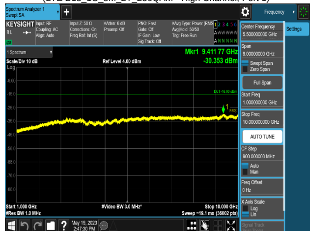
Plot 8-578. Conducted Spurious Emission Plot 1 GHz to 10 GHz
