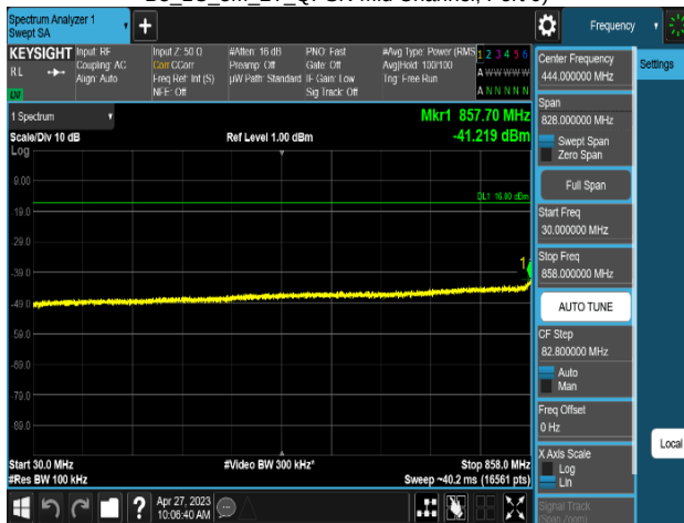
Plot 8-569. Conducted Spurious Emission Plot 30 MHz to 858 MHz (MSR 3NC_DSS B(n)5_1C_10M+NR n5_1C_5M+LTE B5_1C_5M_2T_QPSK-Mid Channel, Port 0)
