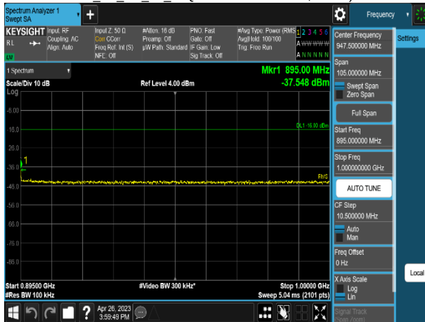
Plot 8-559. Conducted Spurious Emission Plot 895 MHz to 1 GHz (MSR 3C_DSS B(n)5_1C_10M+NR n5_1C_5M+LTE B5_1C_5M_2T_16QAM-Middle Channel, Port 0)
