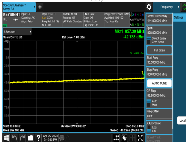
Plot 8-533. Conducted Spurious Emission Plot 30 MHz to 858 MHz (MSR 2NC_NR n5_1C_5M+LTE B5_1C_5M_2T_QPSK-Mid Channel, Port 0)
