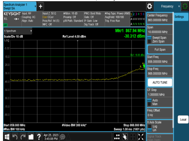
Plot 8-528. Conducted Spurious Emission Plot 858 MHz to 868 MHz (MSR 3C_NR n5_2C_10M+10M+LTE B5_1C_5M_2T_QPSK-Mid Channel, Port 0)
