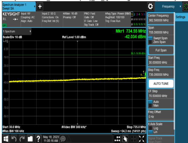
Plot 8-593. Conducted Spurious Emission Plot 30 MHz to 735 MHz (LTE B13 1C_5M+NB-IoT(1IB)_2T_QPSK-High Channel, Port 1)
