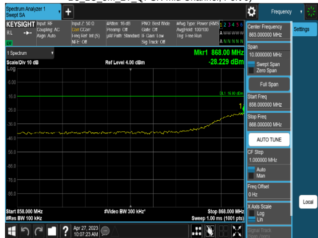
Plot 8-570. Conducted Spurious Emission Plot 858 MHz to 868 MHz (MSR 3NC_DSS B(n)5_1C_10M+NR n5_1C_5M+LTE B5_1C_5M_2T_QPSK-Mid Channel, Port 0)
